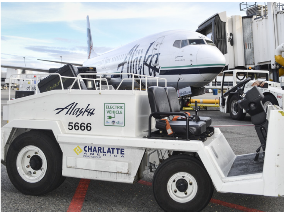
Sea-Tac estimates that there will be 576 charging points throughout the airport to recharge eGSE like this baggage tug when their project is complete. Photo from Western Washington Clean Cities, NREL 34960
