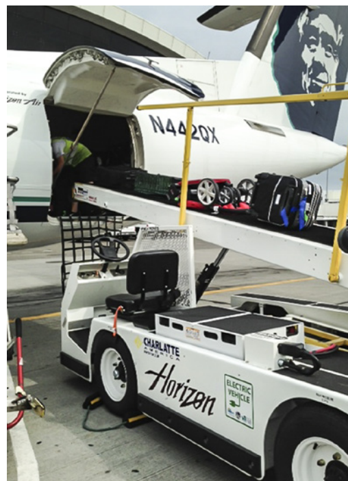
Alaska Air Group currently operates 204 Charlotte America eGSE vehicles, including belt loaders such as this one, which saves the airlines $500,000 annually in fuel costs. Photo from Western Washington Clean Cities, NREL 34959
