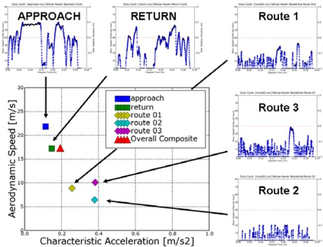
Figure 8: Characterization of the Five OSU Synthetic Cycles
