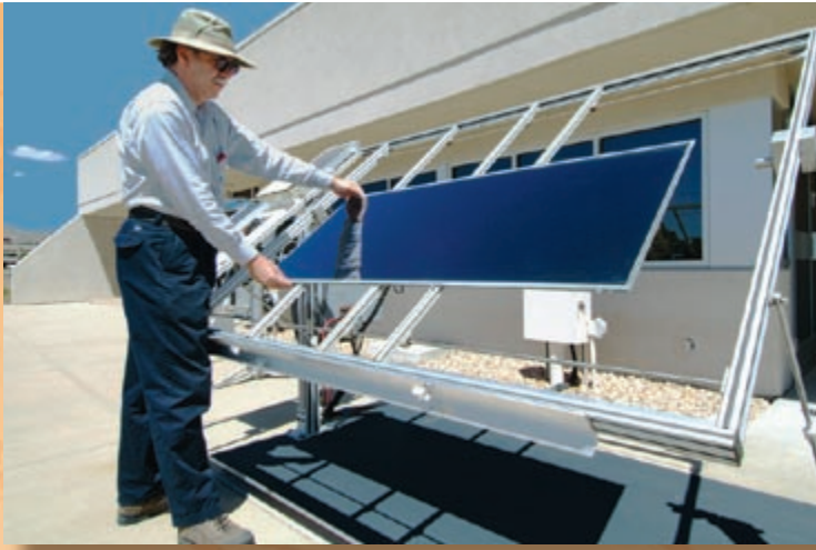
The standard outdoor measurement system is the Laboratory's principal system for measuring module performance under prevailing outdoor conditions.
