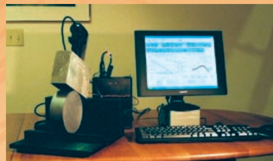
QSSPC System helps increase quality and yield of solar cells.
