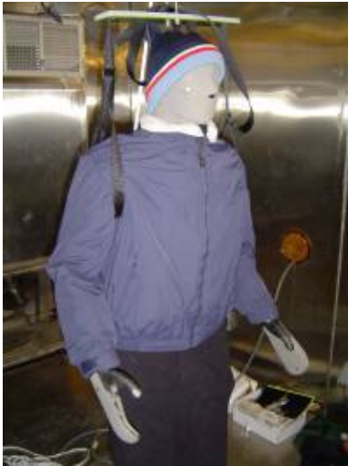
Figure 7. MTNW Reference Clothing Test
