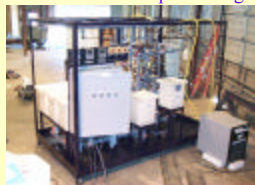
Pilot Scale Electrodialysis System used for industrial processing
