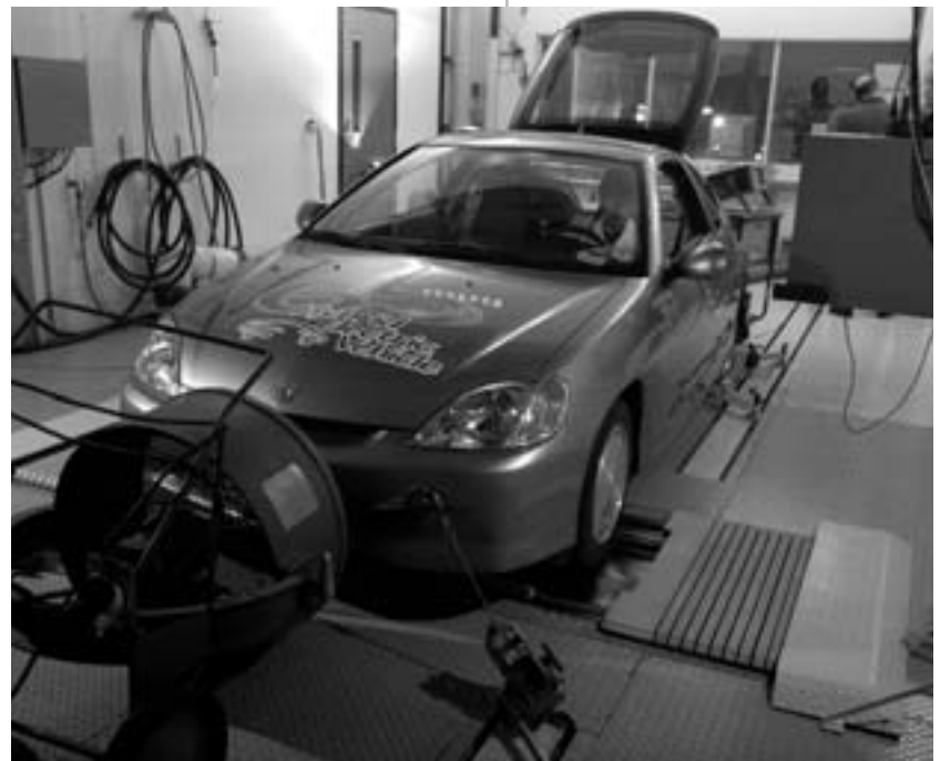
NREL researchers perform dynamometer testing on Honda's Insight hybrid electric vehicle at the Environmental Test Chamber.
