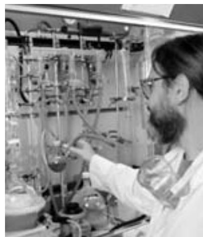
The synthesis of inorganic catalysts are used in the electrocatalytic reduction of carbon dioxide to methanol.
