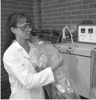
This gas chromatograph measures hydrocarbon emissions from alternative fuel vehicles.
