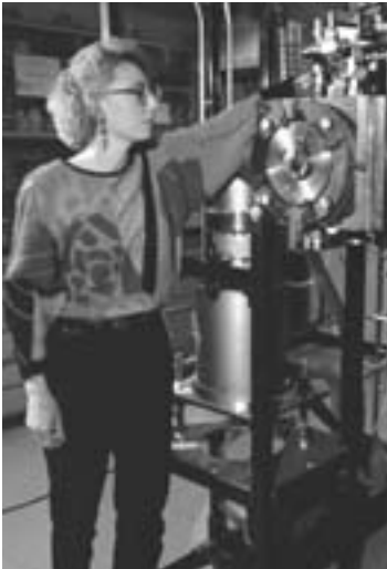
This sophisticated measurement tool developed at NREL brings the laboratory to the power plant. The Transportable Molecular Beam Mass Spectrometer measures elements of the hot-gas stream that cannot be seen with gas chromatography. Analysis of the gas stream helps evaluate cleanup systems at power plants.
