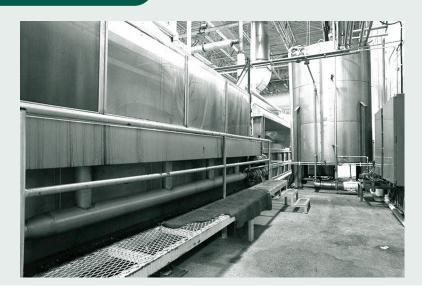
This automated dyebath system includes (from left to right): a carpet dyeing chamber, a holding tank, and a dye analyzer that adjusts dyeing solutions for reuse. This system dramatically reduces energy use, discharged wastes, and overall costs.
