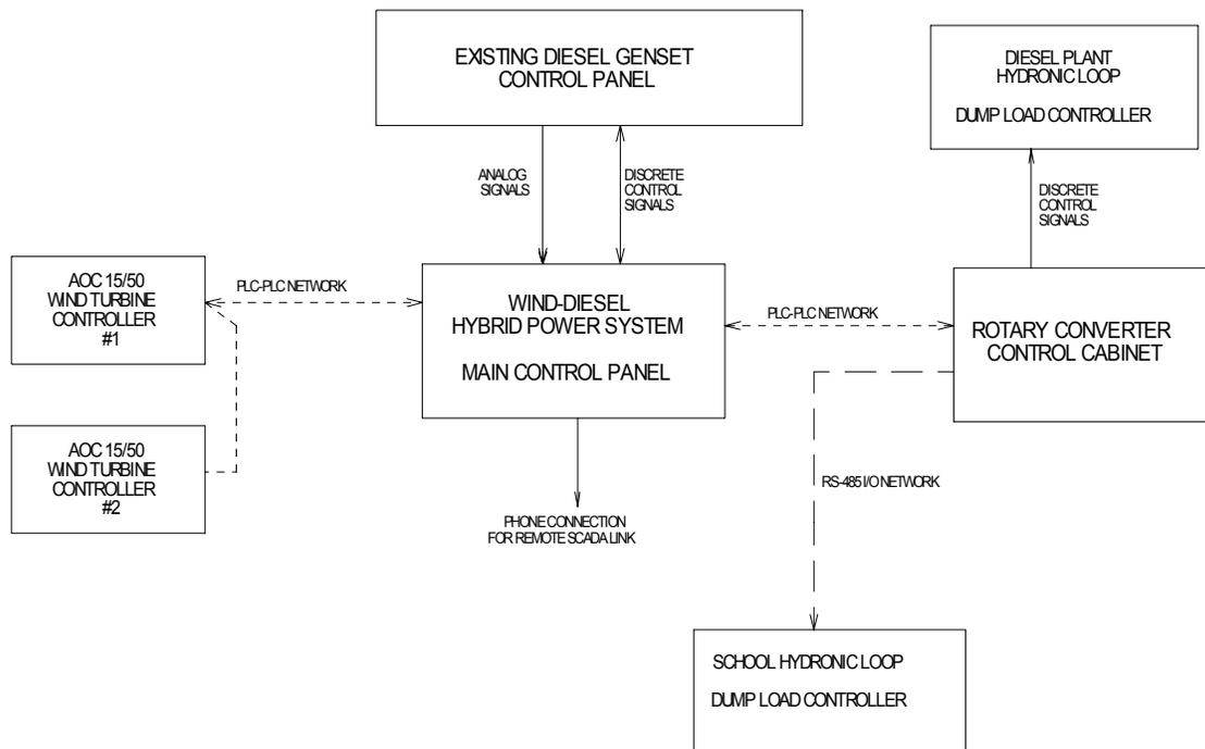
FIGURE 2. WIND-DIESEL SYSTEM COMMUNICATION AND CONTROL DIAGRAM
