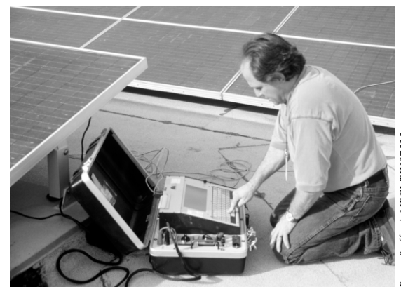
Lorenzo Roybal, an NREL engineer, tests the output of PV panels with an I-V (current-voltage) curve tracer.
