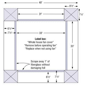
Cut out and discard four corners of fiberglass duct board
