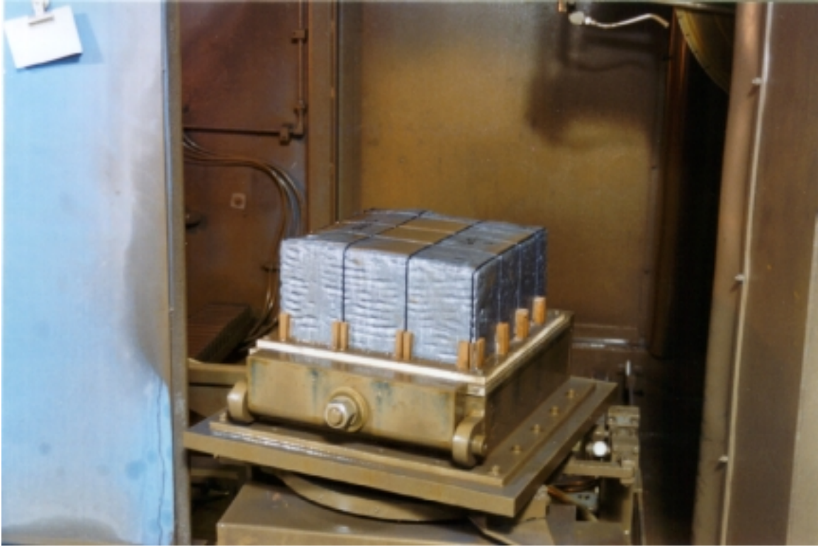
Figure 2 Large “Mongo” Ingot Sized into 9 Bricks
