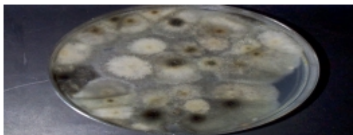
Figure 8. Fungal culture grown from air samples taken from a vehicle's HVAC system
