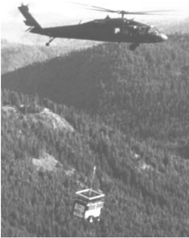
Figure 5. A portable PV genset is helicoptered into the mountains of California (photo courtesy of Live Oak Solar).
