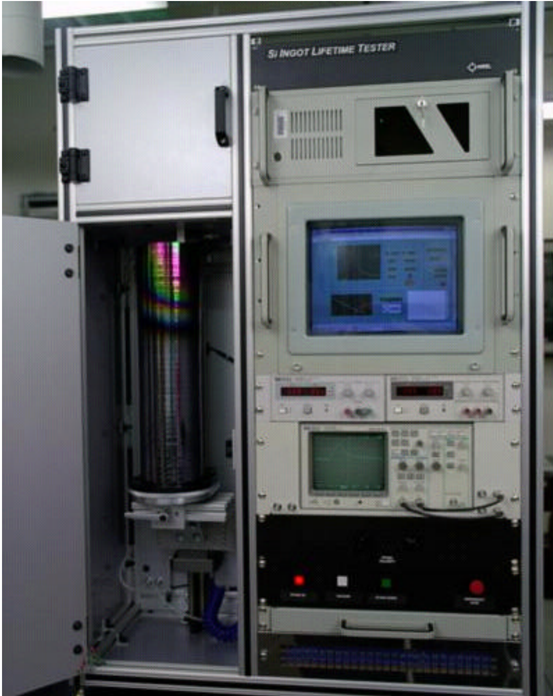
Fig. 2 The Silicon Ingot Lifetime Tester.
