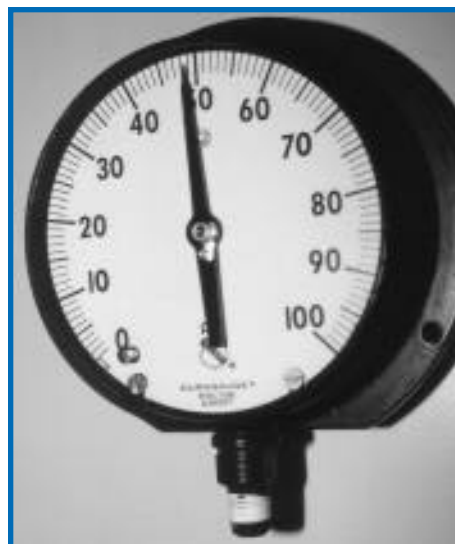
Figure 1. Test pressure gauge.
