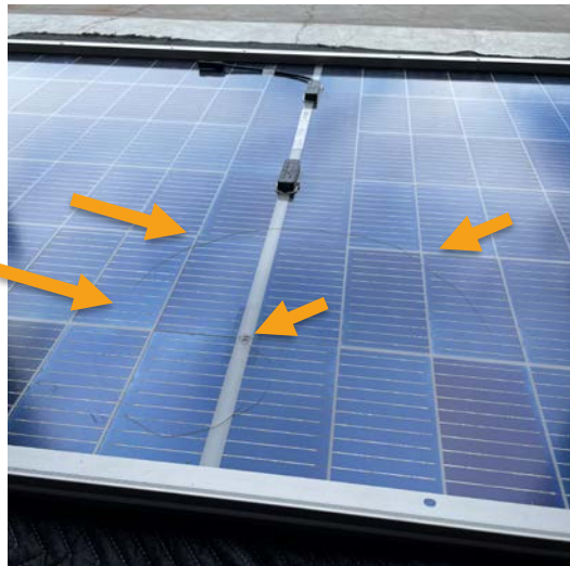
low energy fracture pattern
