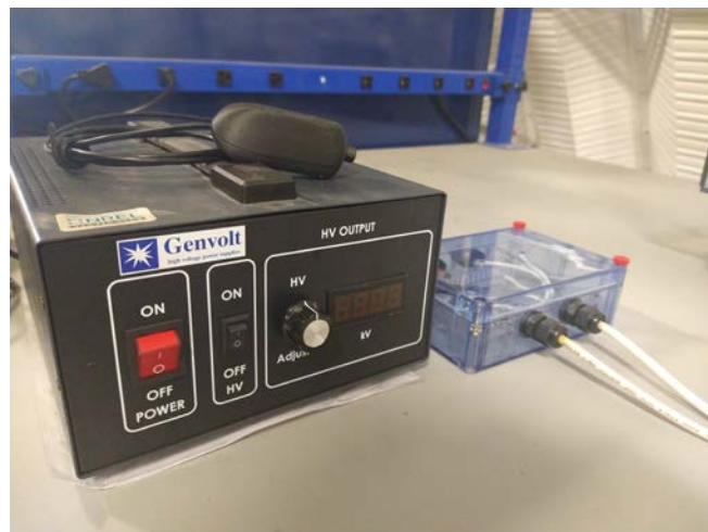
Fig. 5. Genvolt high-voltage power supply with activation switch (left), and high-voltage measurement and actuation circuit in a blue electrical enclosure (right).
