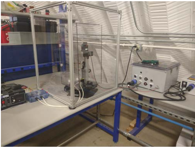
Fig. 6. Full DEEC-Tec testing setup for hyperelastic transducers. From left to right: High-voltage power supply, mechanical actuator and turntable, and NI system and electronics. Not pictured: oscilloscope and 3D scanner setup.
