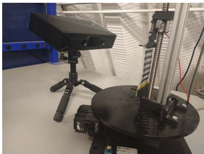
Fig. 4. Polyga Compact S1 scanning setup with turntable. The mechanical actuator and transducer (HASEL) are rotated together to achieve a complete scan while under load.
