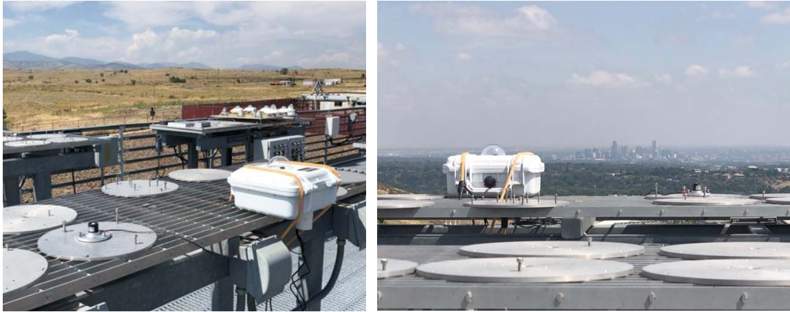
Figure 3: Photographs of the CloudCV sky imager and pyranometer as deployed on the mezzanine of the NREL Mesa Top facility.
