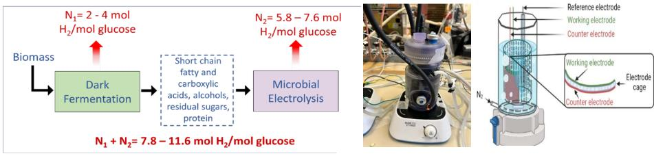
Process flow diagram of the integrated fermentation-MEC process for  $\rm H_2$  production from waste biomass
