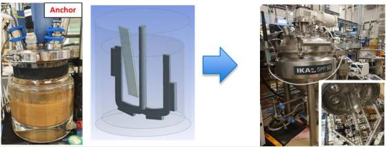
ABPDU fermentation suite is equipped with Rushton and anchor impeller bioreactors, process mass spectrometer, and a 50 L scaleup reactor with customized, high-solids mixing geometry
