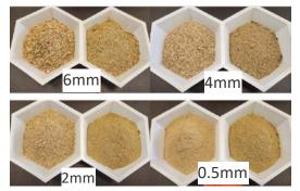
left: before fermentation right: post fermentation (finer particles)
