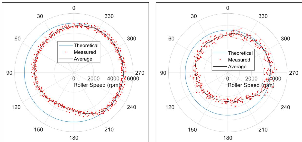
**Figure 6. NU 232 (left, viewed from generator side) and 2326 (right, viewed from generator side) bearing roller speeds at rated power**
