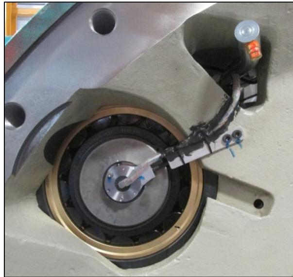
**Figure 3. Slip ring (left) and anti-rotation bracket (right). Photos by Jonathan Keller and Shawn Doner, NREL 49043 and 49752**
