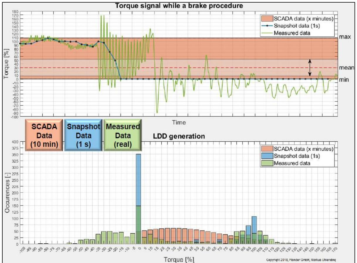
Figure 15. Torque and Load Duration Distribution (LDD) in a braking procedure (Doner 2020)
