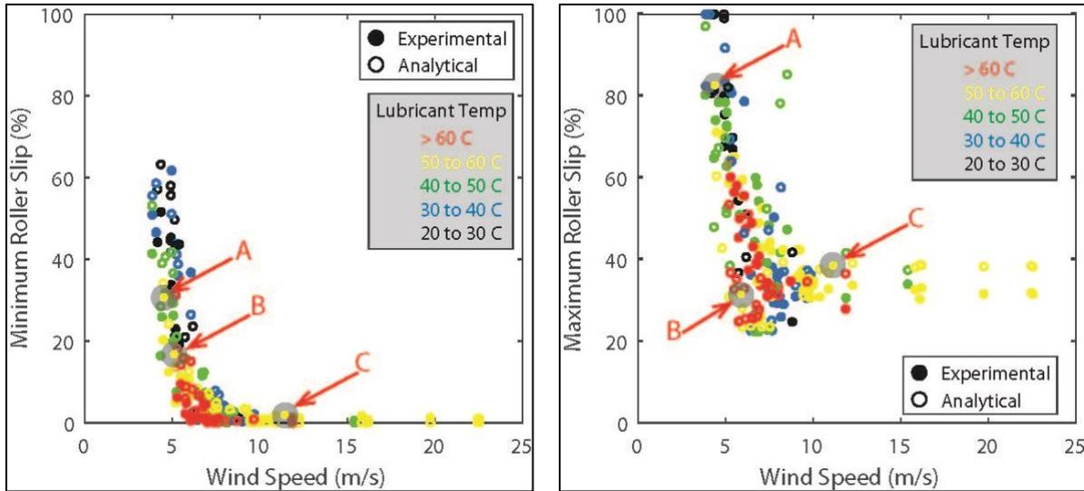
**Figure 10. Minimum (left) and maximum (right) roller slip during normal power production**
