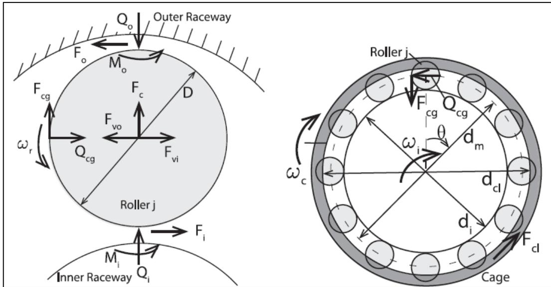
**Figure 9. Free-body diagram of a roller (left) and cage (right) in a CRB**
