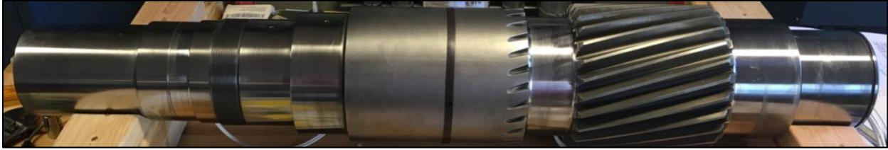
**Figure 2. Machined high-speed shaft. Photo by Jonathan Keller, NREL 49040**
