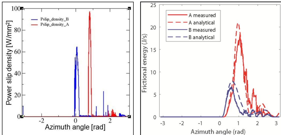
**Figure 11. Power slip density (left) and cumulative frictional energy (right) for 80% torque**
