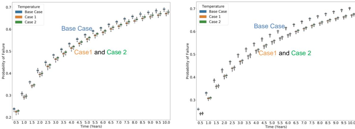
**Figure 13. Effect of lubricant temperature on probability of failure for (left) bearing A and (right) B**
