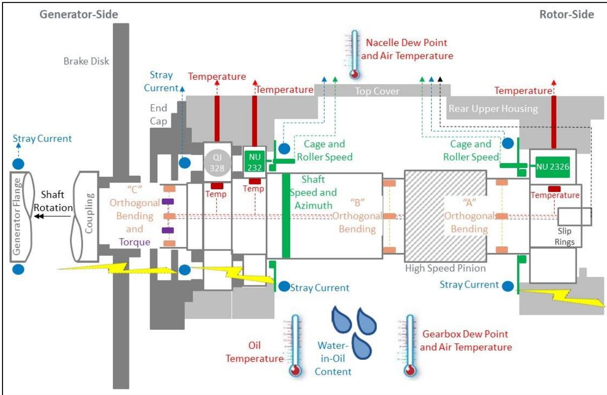
Figure 1. High-speed-shaft instrumentation schematic
