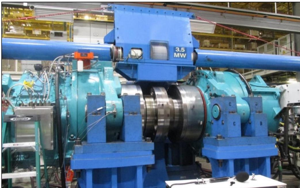
**Figure 5. Production acceptance load test. Photo by Shawn Doner, NREL 50080**
