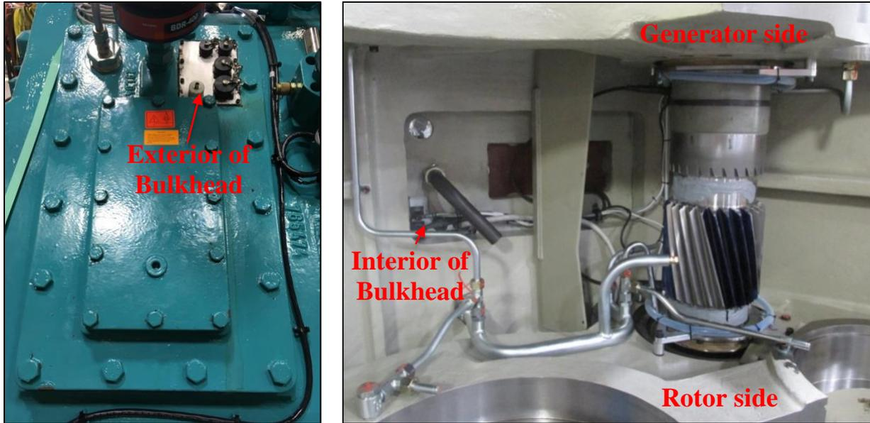
**Figure 4. Exterior (left) and interior (right) bulkheads. Photos by Jonathan Keller and Shawn Doner, NREL 49049 and 49750**
