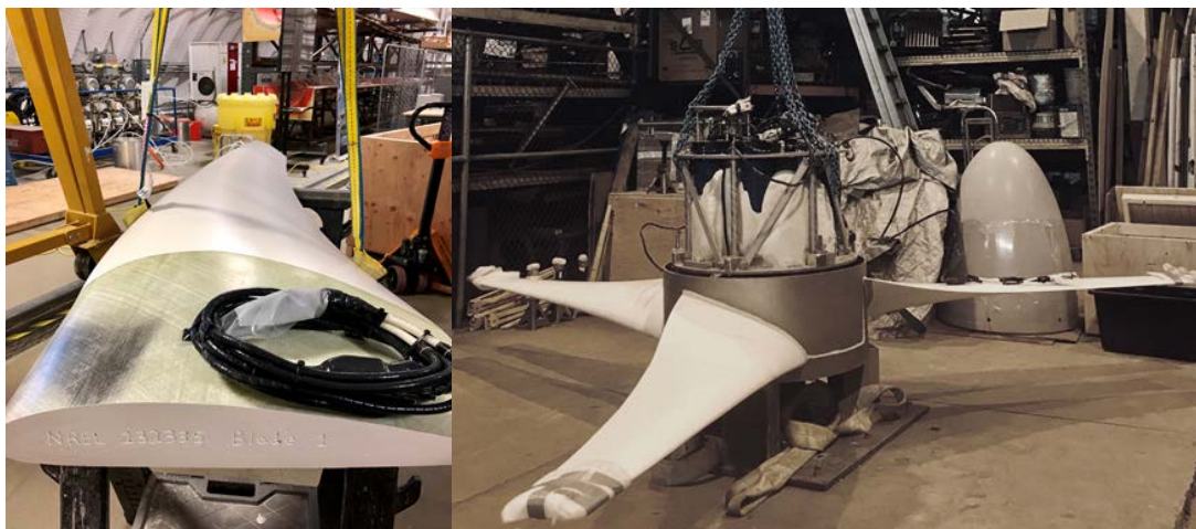
Figure 4. Completed thermoplastic blade (left) and thermoplastic blades in the Verdant Power hub ready for turbine assembly (right).
