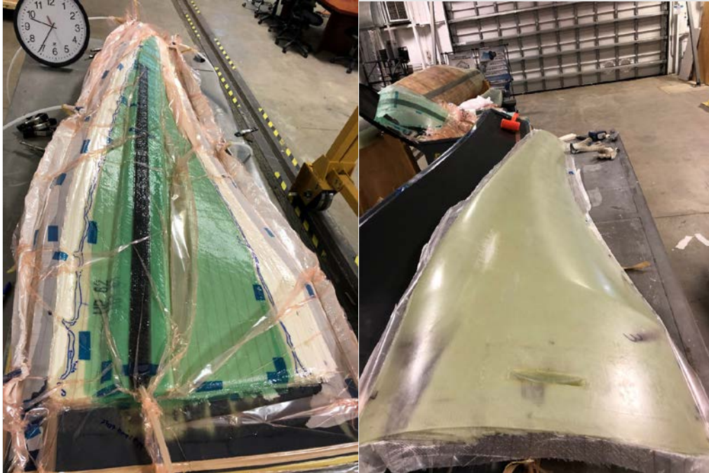
Figure 3. High-pressure thermoplastic blade skin mid-infusion (left) and completed high-pressure skin (right).
