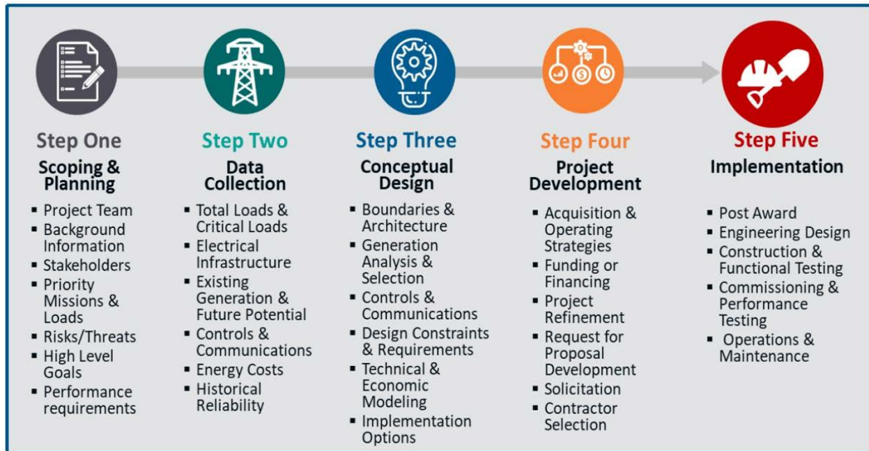
Figure 1. NREL's microgrid design process
