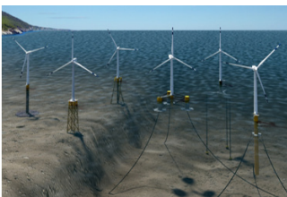
Offshore wind turbine substructure types. From left: monopile, jacket, inward battered guide, semisubmersible, tension-leg platform, and spar. Illustration by Joshua Bauer, NREL
