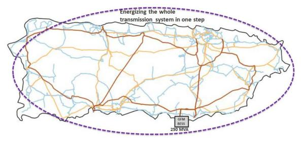
Figure 222. Energizing the entire transmission network by one step with all loads disconnected
