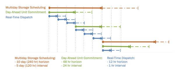
Figure 147. Illustration of PCM simulation configuration
