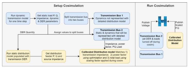
Figure 216. T&D cosimulation setup
