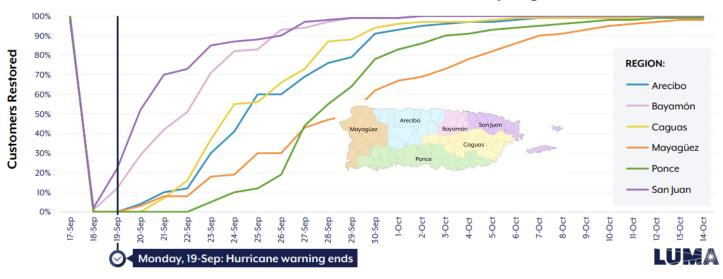
Figure 15. Power restoration over time after Hurricane Fiona by region of Puerto Rico Source: LUMA (2022)
