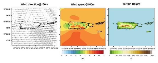
Figure ES-10. Maps of 20-yr mean wind speeds, wind direction at 160 m, and terrain height for Puerto Rico
