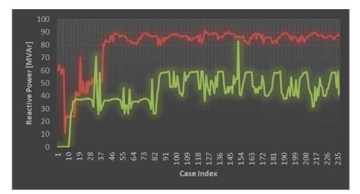
Figure 174. Capacitive reactive compensation needs, at two locations (green and red curves), for each hour of one week of August 2028, 3LS scenario
