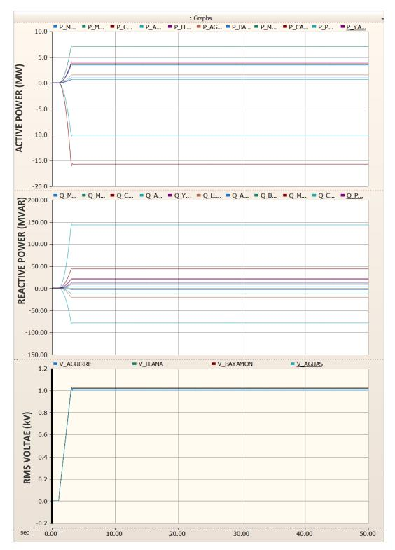
Figure 223. Energizing the entire transmission system with GFM BESS: Active (upper graph) and reactive (middle graph) power, system voltages (lower graph)
