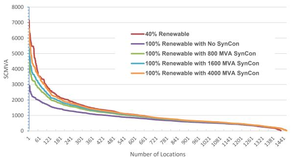
Synchronous Condensers Capacity at Existing Plant Locations
