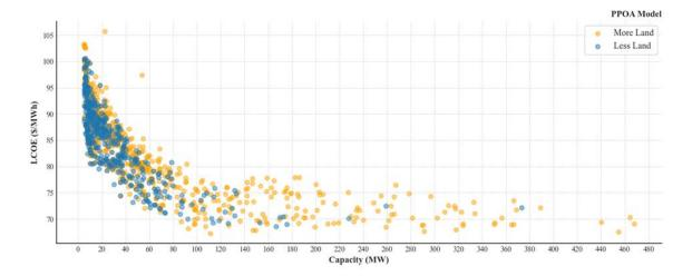
Figure ES-11. Total LCOE by plant capacity in 2030 for expected levels of technology innovation
