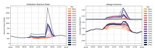
Figure 290. Substation delivered reactive power of Feeder 1 (left) and voltage extremes (right) from the 3LS distributed storage simulation
