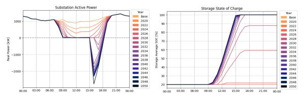
Figure 288. Substation delivered active power of Feeder 1 (left) and distributed storage SOC (right) from the 3LS distributed storage simulation
