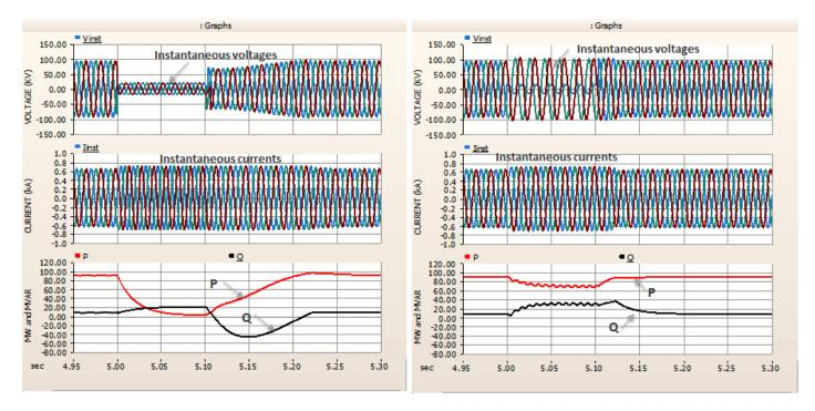
Figure 195. Simulated LVRT performance of 100-MW PV plant for (left) 100 ms three-phase voltage fault and (right) 100 ms single-phase voltage fault at 115-kV POI
