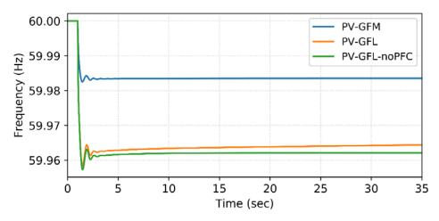
Figure 202. Frequency response to 90-MW outage for 830-MW GFM batteries and GFM and GFL utility-scale PV
