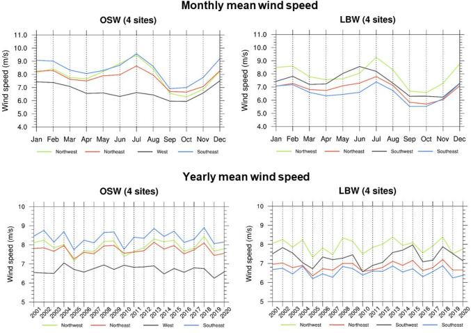
Figure 55. Monthly and annual mean wind speeds for offshore wind and land-based wind sites
