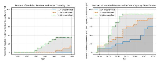
Figure 252. Percentage of modeled feeders with overloading line (left) and service transformer (right) violations in the uncontrolled simulation
