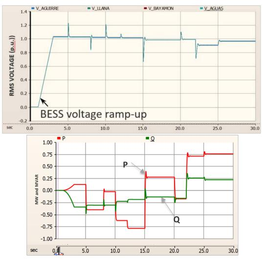
Figure 220. Simulation of black-start energization of 230-kV transmission segments from single BESS
