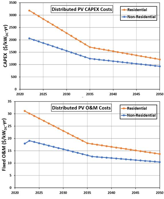
Figure 117. Distributed PV CapEx and O&M cost projections
