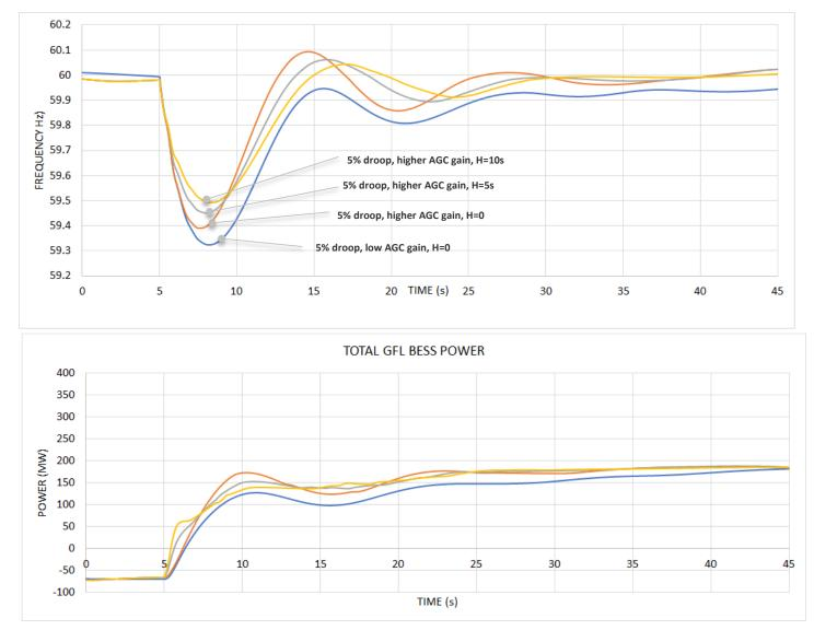
Figure 197. LUMA frequency response (upper graph) and active power of all Tranche 1 BESS (lower plot) operating in GFL mode with different controls
