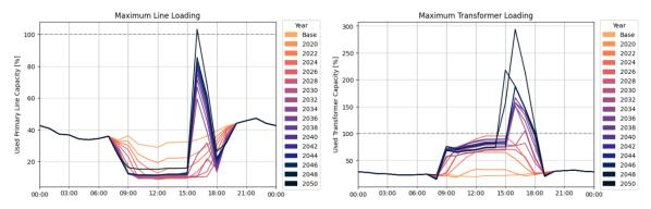
Figure 289. Maximum line loading (left) and transformer loading (right) of Feeder 1 from the 3LS distributed storage simulation
