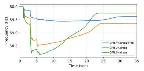
Figure 201. System frequency for severe bus fault contingency for GFM inverters and droopbased FFR
