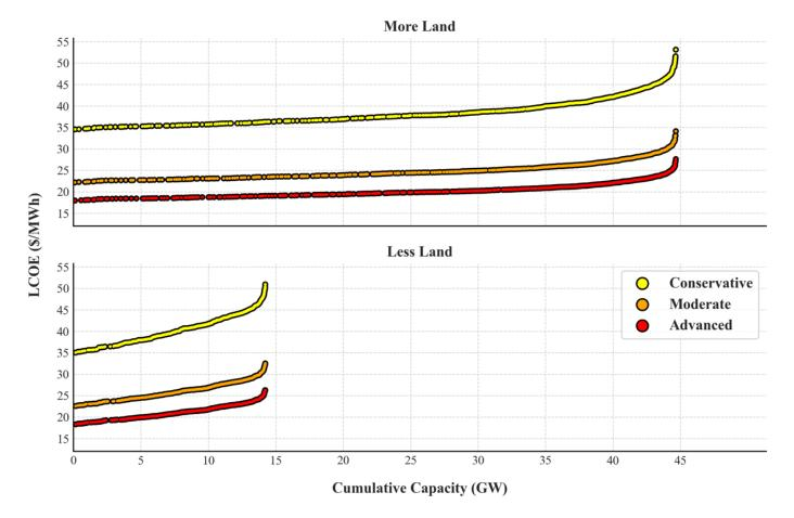
Figure 45. LCOE by cumulative capacity for the 2030 Moderate Technology scenario for both land access variations using the Simple FCR LCOE method
