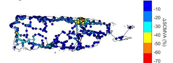
Figure 184. Change in short circuit capacity 38-kV system
