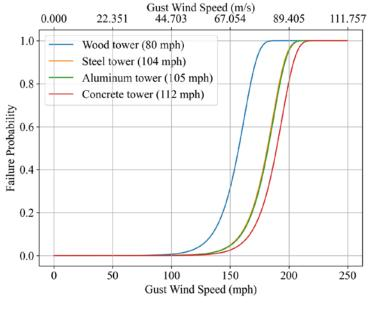
Figure 224. Fragility curves for electrical towers
