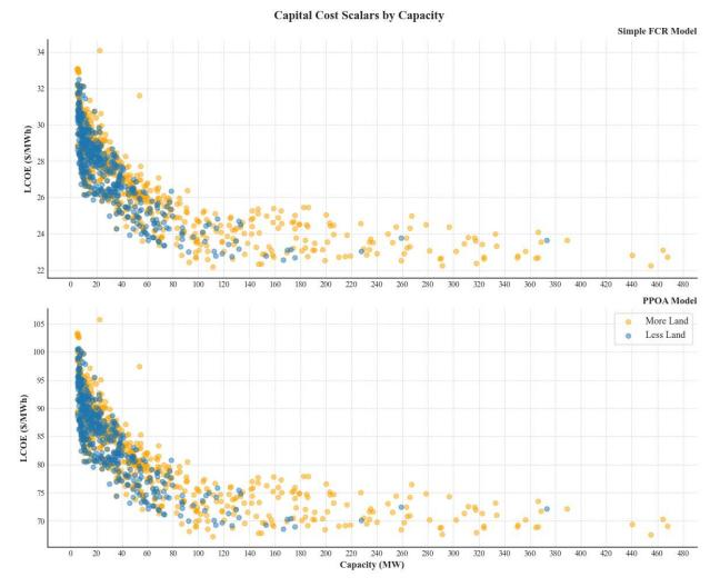
Figure 44. Total LCOE by plant capacity for the 2030 ATB Moderate Technology scenario
