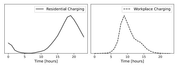
Figure 84. Two light-duty EV unmanaged charging profiles assumed to occur at residential locations (left) and places of work (right)
