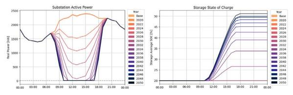
Figure 271. Substation delivered active power (left) and storage fleet SOC (right) from Feeder 19 during the 2LS utility storage simulation
