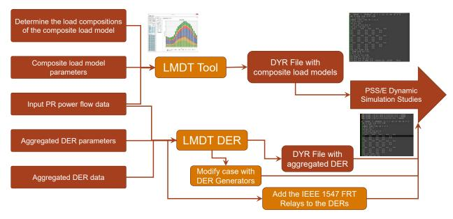
Figure 204. PSS/E model augmentation to include dynamic models for loads, DERs and FRT relays to capture inverter's FRT capability
