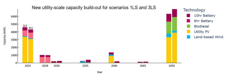
Figure 141. Year-by-year new utility-scale capacity build-out for scenarios 1LS and 3LS
