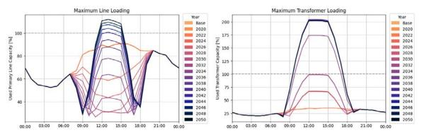
Figure 261. Maximum line (left) and transformer (right) loading of Feeder 19 during the 2LS uncontrolled simulation
