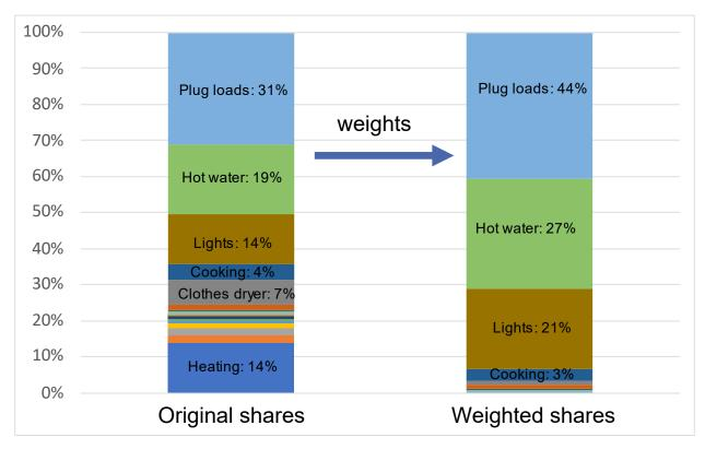
ResStock Miami: Share of end uses excluding cooling, refrigerator, and ceiling fans
