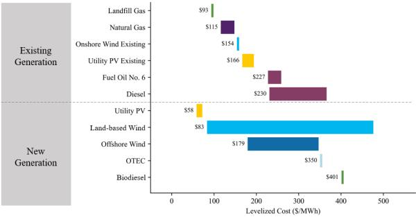
Figure 134. Levelized cost of eletricity by technology in 2035 (costs in 2021 real dollars)
