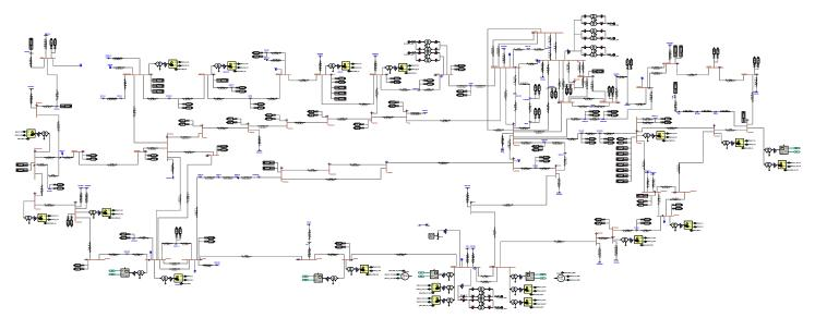
Figure 193. PSCAD model of LUMA grid: 115-kV transmission system layer with interconnected Tranche 1 PV and BESS plants
