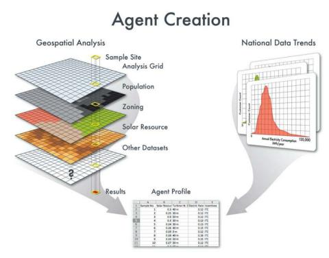
Figure 114. The fundamental design of dGen—multiple spatial layers from peer-reviewed data sets and complementary software—is used to build agents, which are statistical representations of the underlying data.
