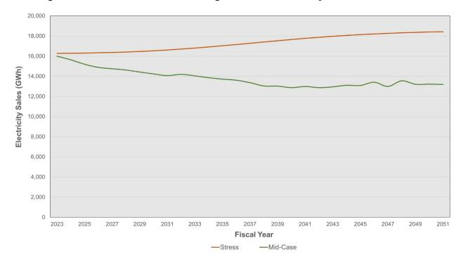
Figure 111. PR100 electric load projections: Mid case and Stress variations for all of Puerto Rico (FY23–FY51)
