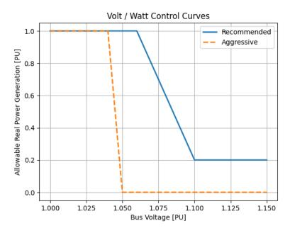
Figure 246. Control curves for recommended and aggressive Volt/Watt control
