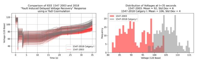
Figure 217. Comparison of IEEE 1547-2003 and IEEE 1547-2018 FIDVR using T&D cosimulation
