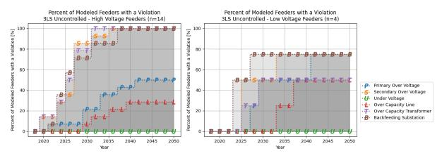
Figure 303. Percentage of high (left) and low (right) voltage feeders with a violation in the 3LS uncontrolled simulation
