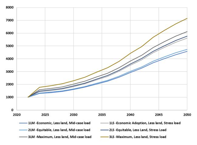
Figure 124. Cumulative distributed battery size (MWh) by scenario
