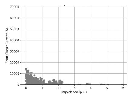
Figure 180. 100% Renewable case fault current contribution of all generators
