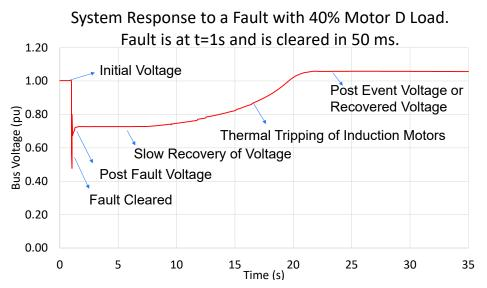
Figure 207. A FIDVR event for a bus fault with 40%  $1 - \phi$  induction motor load modeled through composite load models
