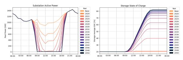
Figure 301. Substation delivered active power (left) and storage fleet SOC (right) from Feeder 1 during the 3LS combination storage simulation.
