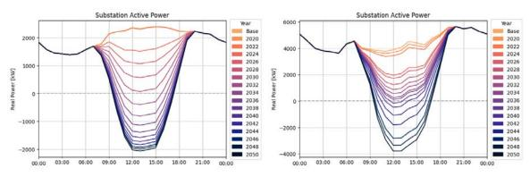
Figure 259. Substation delivered active power of Feeder 19 (left) and Feeder 7 (right) of the 2LS uncontrolled simulation
