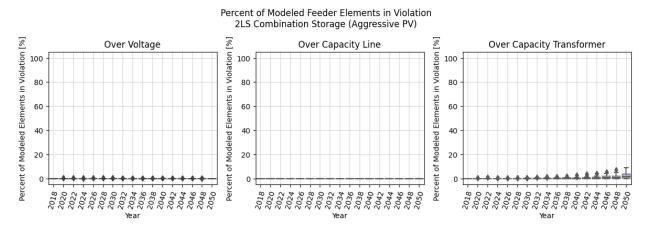
Figure 297. Percentage of feeder elements in violation for the 2LS combination storage simulation
