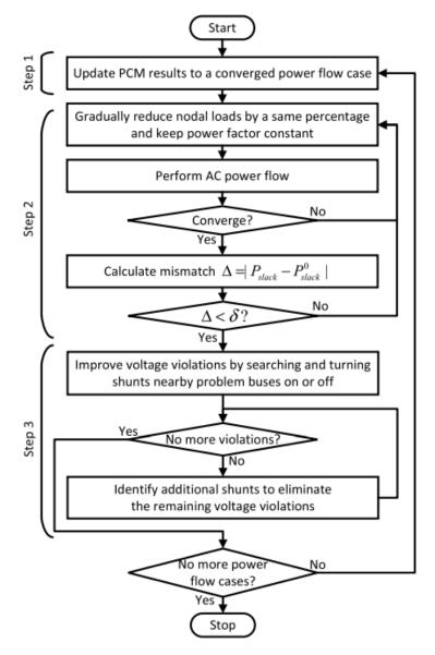
Figure 171. Proposed procedure to convert a DC-converged power flow case from PCM results to an AC-converged power flow case
