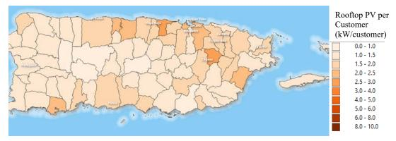
Figure ES-17. Year 2050 rooftop PV capacity per customer for Scenario 1 with Mid case load (1LM)
