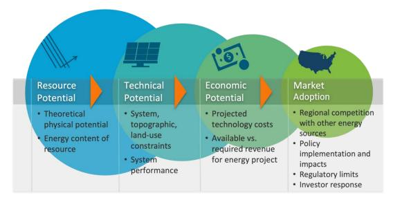
Figure 25. Levels of renewable energy potential analysis, starting with the theoretical potential provided by a region's atmospheric resource and progressively refining this estimate with technical, economic, and market considerations
