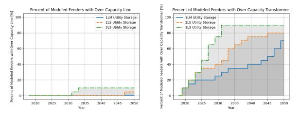
Figure 264. Percentage of modeled feeders with overloading violations in the utility storage simulation
