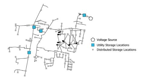
Figure 241. Example of utility and distributed storage placement on a distribution feeder
