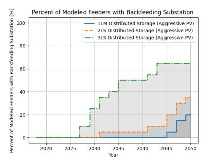
Figure 279. Percentage of modeled feeders with backfeeding violation in the distributed storage simulation
