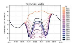
Figure 272. Maximum line loading from Feeder 19 during the 2LS utility storage simulation
