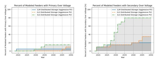
Figure 280. Percentage of modeled feeders with primary and secondary voltage violations in the distributed storage simulation
