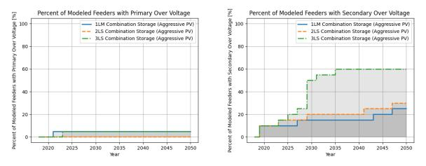
Figure 292. Percentage of modeled feeders with primary and secondary voltage violations in the combination storage simulation
