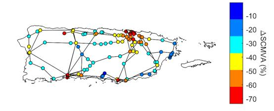
Figure 185. Change in short circuit capacity high-voltage system
