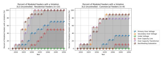
Figure 305. Percentage of residential (left) and commercial (right) class feeders with a violation in the 3LS uncontrolled simulation
