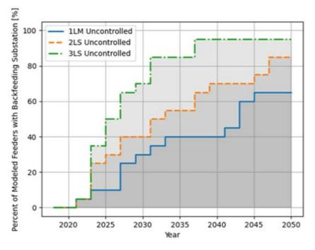
Figure ES-25. Percentage of feeders with back-feeding substations
