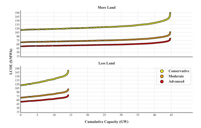
Figure 46. LCOE by cumulative capacity for the 2030 Moderate Technology scenario for both land variations using the PPOA model
