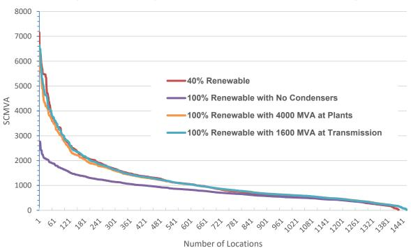
Capacity and Location of Synchronous Condensers to Match 2026 Grid Strength
