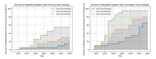
Figure 251. Percentage of modeled feeders with primary and secondary voltage violations in the uncontrolled simulation
