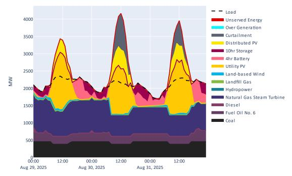
Figure 149. Sample dispatch for 1LM scenario using the PR100 operational scheduling configuration
