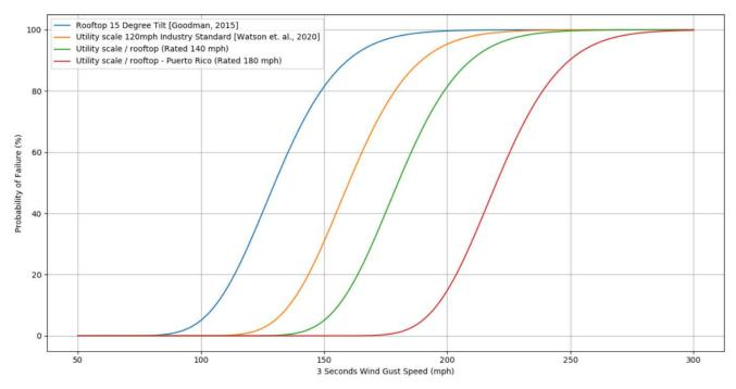
Figure 225. Fragility curves for rooftop and utility solar
