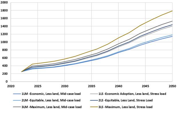
Figure 123. Cumulative distributed battery storage power (MW) by scenario
