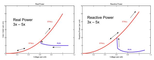
Figure 208. Active power (left) and reactive power (right) versus the voltage for the normal and stalled operation for the 1- $\phi$  induction motor
