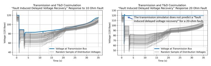
Figure 218. Comparison of FIDVR using only a transmission simulation and using T&D cosimulation
