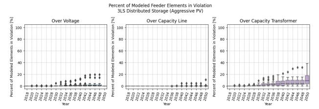
Figure 287. Percentage of feeder elements in violation for the 3LS distributed storage simulation
