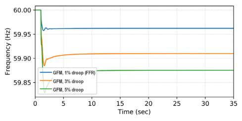
Figure 200. System frequency for single contingency of generation tripping for GFM inverters and droop-based FFR
