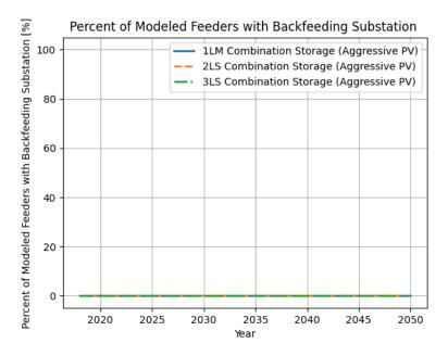
Figure 291. Percentage of modeled feeders with backfeeding violation in the combination storage simulation
