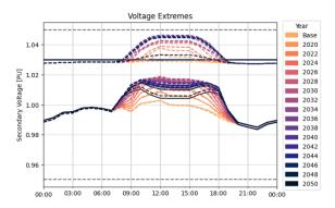
Figure 302. Primary (solid) and secondary (dashed) voltage extremes of Feeder 1 during the 3LS combination storage simulation
