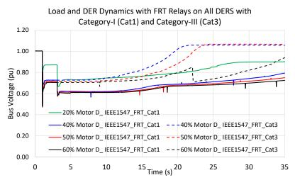
Figure 213. Impact of DER inverter's IEEE 1547 FRT capability for Cat 1 and Cat 3 with varying load compositions
