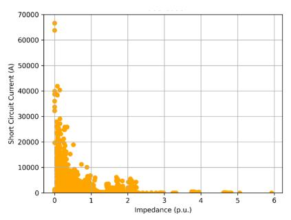
Figure 179. 100% Conventional case fault current contribution of all generators
