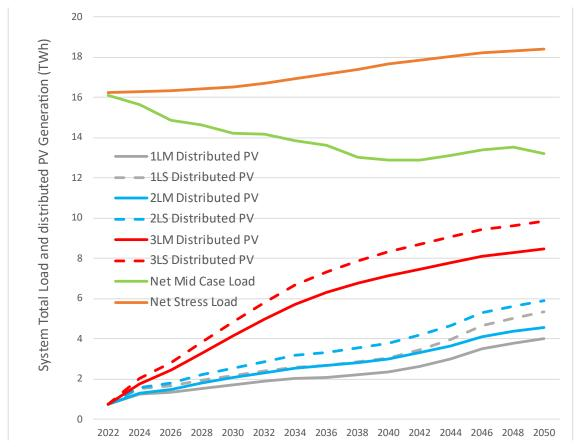
Figure ES-16. Rooftop PV generation across scenarios and Puerto Rico load forecasts plotted to demonstrate the fraction of annual load met by distributed generation
