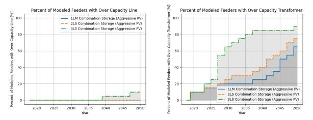
Figure 293. Percentage of modeled feeders with overloading violations in the combination storage simulation
