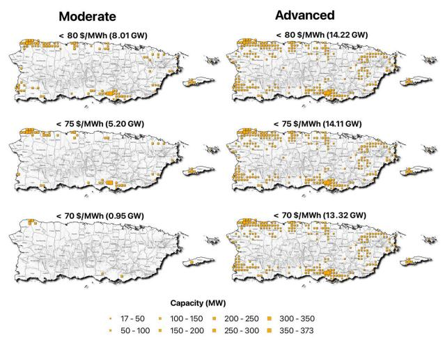
Figure 50. Remaining capacity under different cost thresholds for the 2030 Less Land, Moderate Technology, and Advanced Technology scenarios using the PPOA LCOE model
