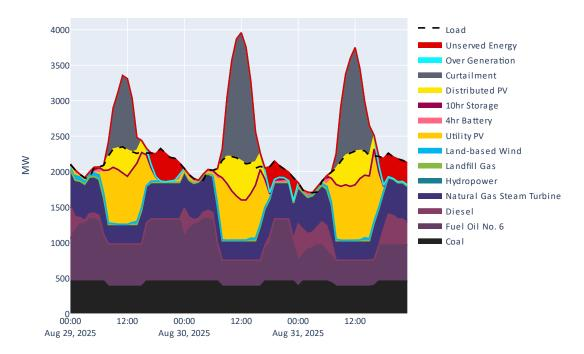
Figure 148. Sample dispatch for 1LM scenario using common operational scheduling configuration (not used for PR100 results)
