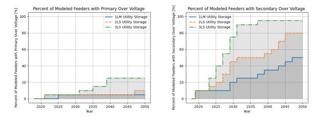
Figure 263. Percentage of modeled feeders with primary and secondary voltage violations in the utility storage simulation
