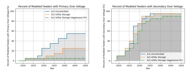
Figure 273. Percentage of modeled feeders with primary and secondary voltage violations using expected and aggressive PV inverter controls
