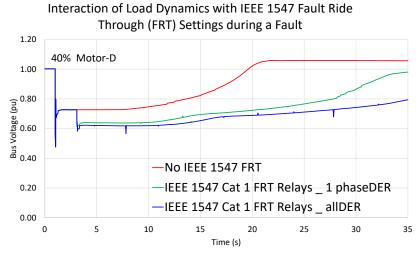
Figure 211. Interaction of load and DER dynamics with FRT capability
