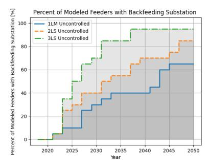
Figure 250. Percentage of modeled feeders with backfeeding violation in the uncontrolled simulation
