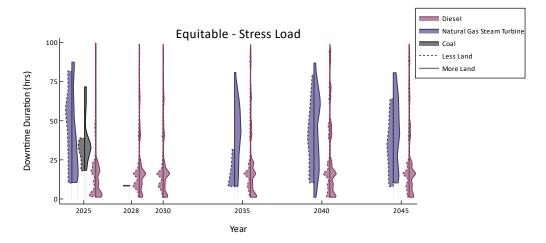
Figure H-18. Fossil-fueled generator downtime duration for Equitable Adoption scenarios under the Stress Load variation (2\*S)
