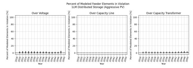
Figure 283. Percentage of feeder elements in violation for the 1LM distributed storage simulation
