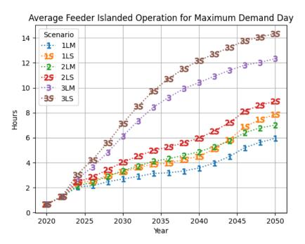
Figure 309. Average hours fully charged utility storage simulation could serve a feeder assuming maximum day demand and no additional charging of storage
