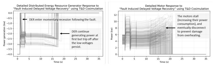
Figure 219. DER generator and motor response to FIDVR
