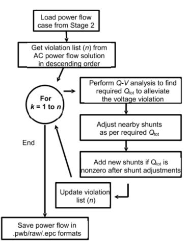
Figure 172. Reactive power planning to improve voltage profile
