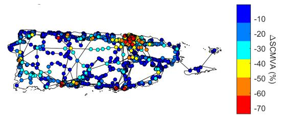
Figure 183. Change in short circuit capacity system-wide
