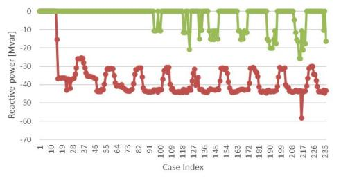
Figure 175. Inductive reactive compensation needs, at two locations (green and red curves), for each hour of one week of August 2028, 3LS scenario
