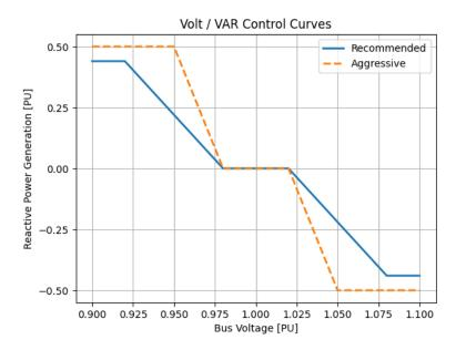
Figure 245. Control curves for recommended and aggressive Volt/VAR control
