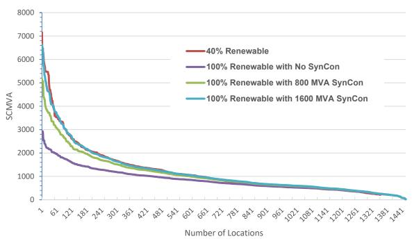
Figure 188. Synchronous condenser sensitivity at transmission
