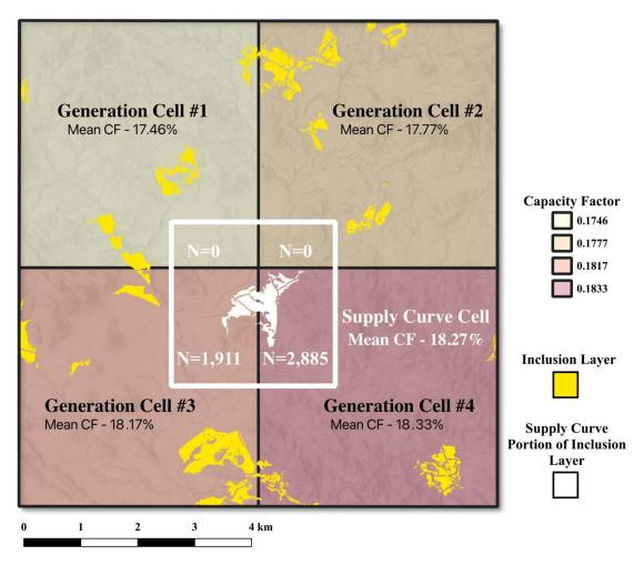
Figure 32. Visualization of the aggregation process for reV Generation capacity factors within a supply curve cell
