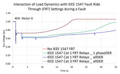
Figure 212. Interactions of load dynamics and DER IEEE 1547 FRT capability for Cat 1 and Cat 3
