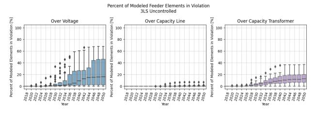
Figure 258. Percentage of feeder elements in violation for the 3LS uncontrolled simulation
