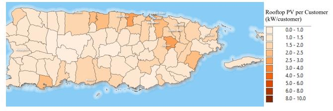
Figure 128. 2050 Rooftop PV capacity per customer for Scenario 1 with Mid case load (1LM)
