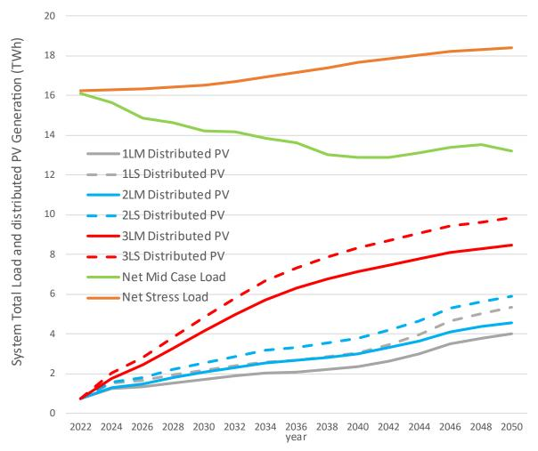
Figure 122. Rooftop PV generation in six scenario variations compared with net load forecast variations (Mid case and Stress)
