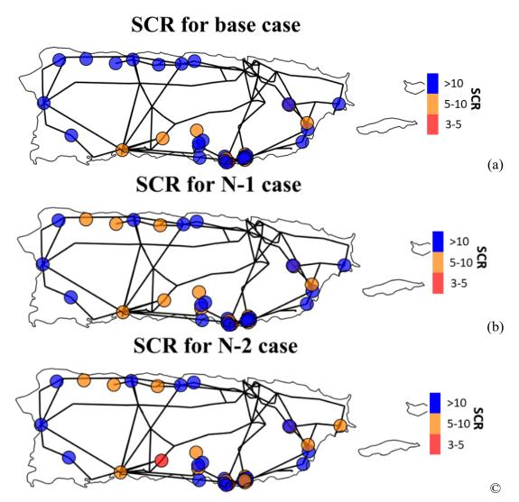
Figure 189. SCR for 100% renewable case (a) without any contingencies (b) for most critical line contingency (N-1) corresponding to each POI (c) for second-most critical line contingencies (N-2) corresponding to each POI
