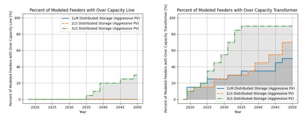
Figure 281. Percentage of modeled feeders with overloading violations in the distributed storage simulation
