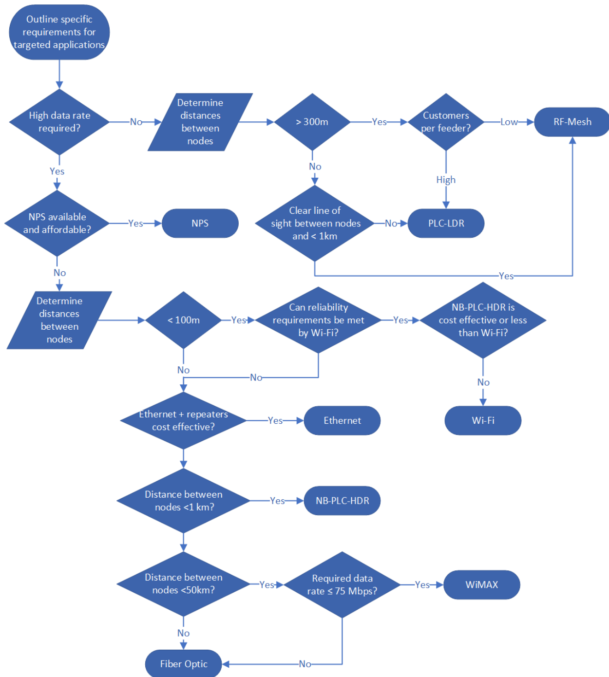
Figure 14. Design methodology for the selection of common physical layers. Cost constraints and benefits will vary by location. High data rate requirements may add constraints.
