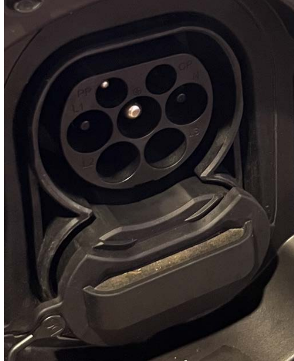
Figure 3. Vehicle side of a Mennekes Type 2 connector, as required for AC charging stations by IEC 62196.
