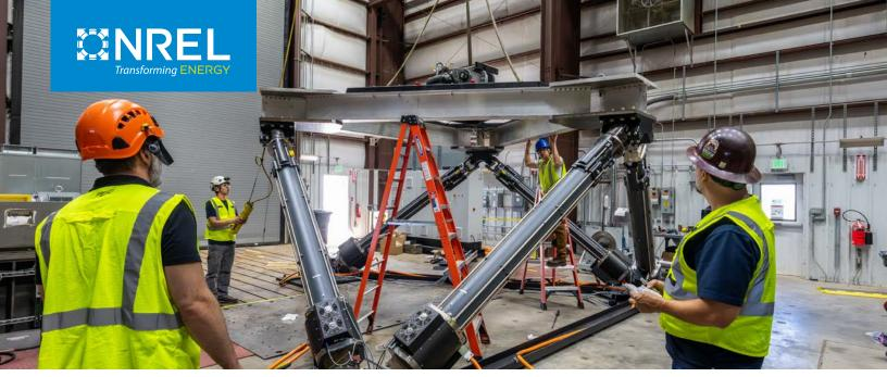
Researchers have been using the large-amplitude motion platform to validate wave energy converter devices, such as the HERO WEC, NREL's first wave-powered desalination system. *Photo by Josh Bauer, NREL*
