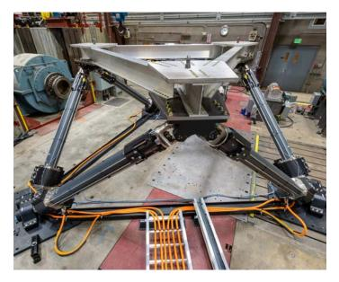
The lab's large-amplitude motion platform, or LAMP, can mimic ocean motions, including waves up to 8 feet high, and support devices weighing about as much as a small recreational vehicle. *Photo by Bryan Bechtold, NREL*
