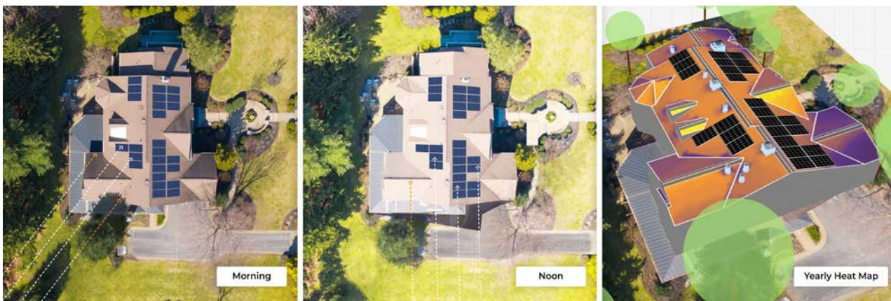
Figure 1. Overview of shading imagery in the Solargraf tool. Image from Enphase Energy
