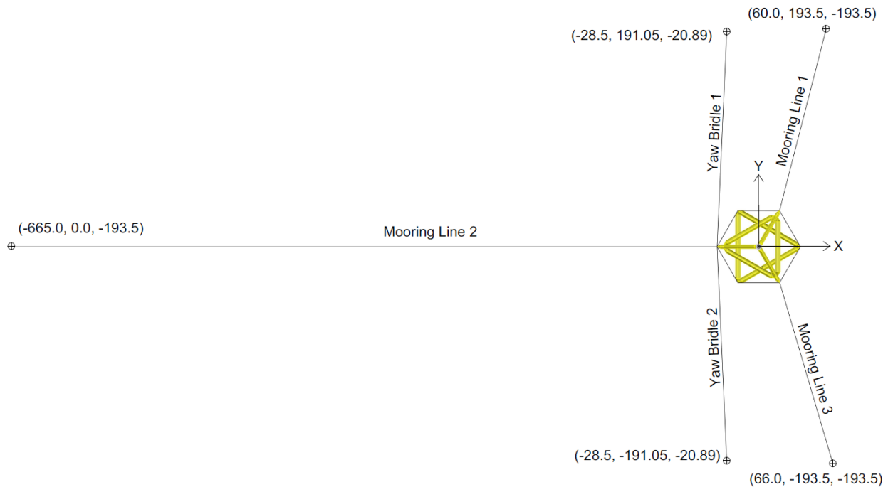
Figure 20. Mooring arrangement with full-scale anchor locations
