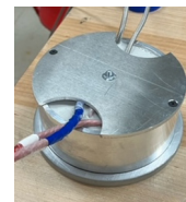
Manufactured inductor for current source inverter for University of Wisconsin's integrated traction drive. Image by University of Wisconsin
