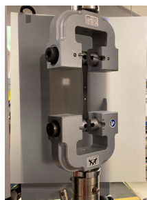
Sample from SNL undergoing tensile testing. Photo by Emily Cousineau, NREL (left). Comparison of samples with different loading showing the change in mechanical properties. Each entry is the average of three samples (right).
