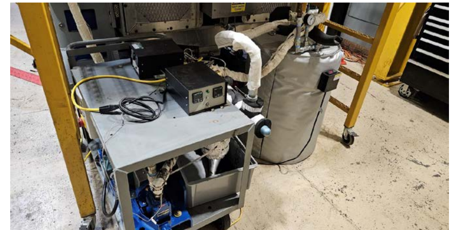
55-gallon heavy fuel oil supply system
