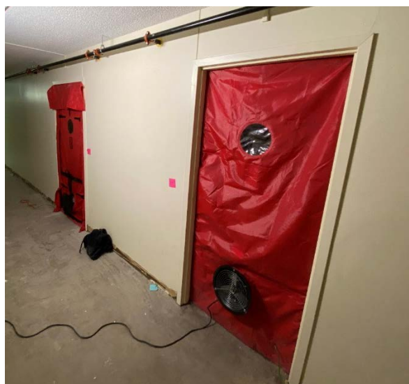
Figure 48. Two-fan guarded zone test of side-by-side units
