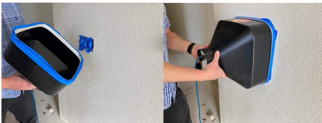
Figure 6. Leakage measurement tool used to measure leakage of light switch
