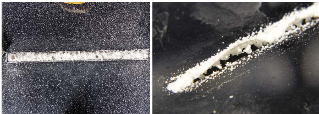
Figure 64. Failed seals occurring in the middle (left) and edge (right) of leak
