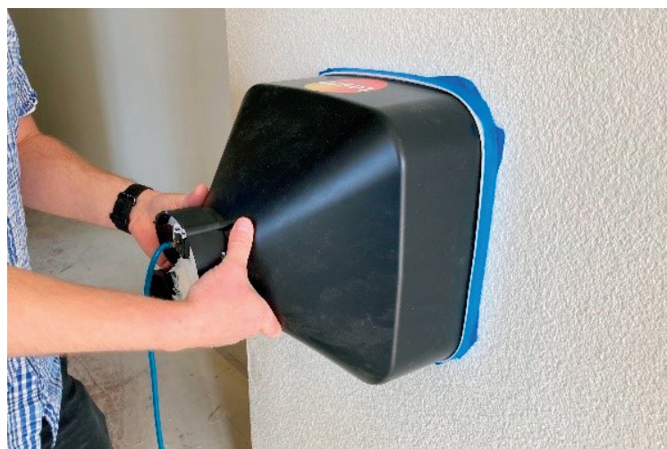
Leakage measurement tool used to measure leakage around a light switch. Photo by the authors
