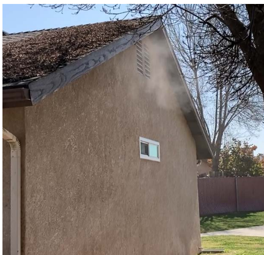
Figure 53. Sealant fog moving out of attic from a gable vent
