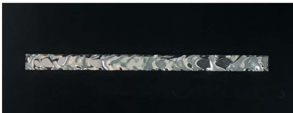
Figure 61. Incomplete ABF23 seal formed on 1/4-in. slot leak showing improved transparency after several days
