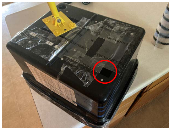
Figure 5. Leakage measurement tool used by CEE staff
