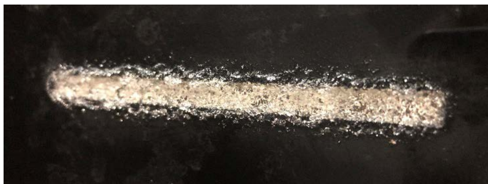
Figure 60. ABF23 seal formed on 1/4-in. slot leak
