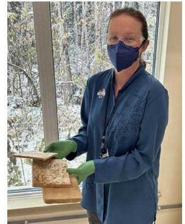
Top: Researcher Robbin Garber-Slaght with samples of insulation grown from mycelium and cellulose. Left: The circular process of producing insulation from insect-killed trees to construct carbon-neutral buildings. Photo by Molly Rettig, NREL; Illustration by Milena Coakley, NREL
