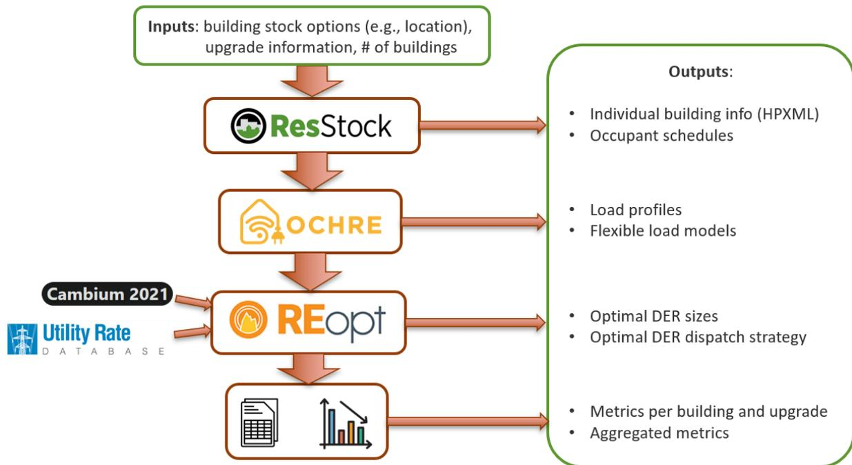
**Figure 3. Visual representation of analysis workflow**
