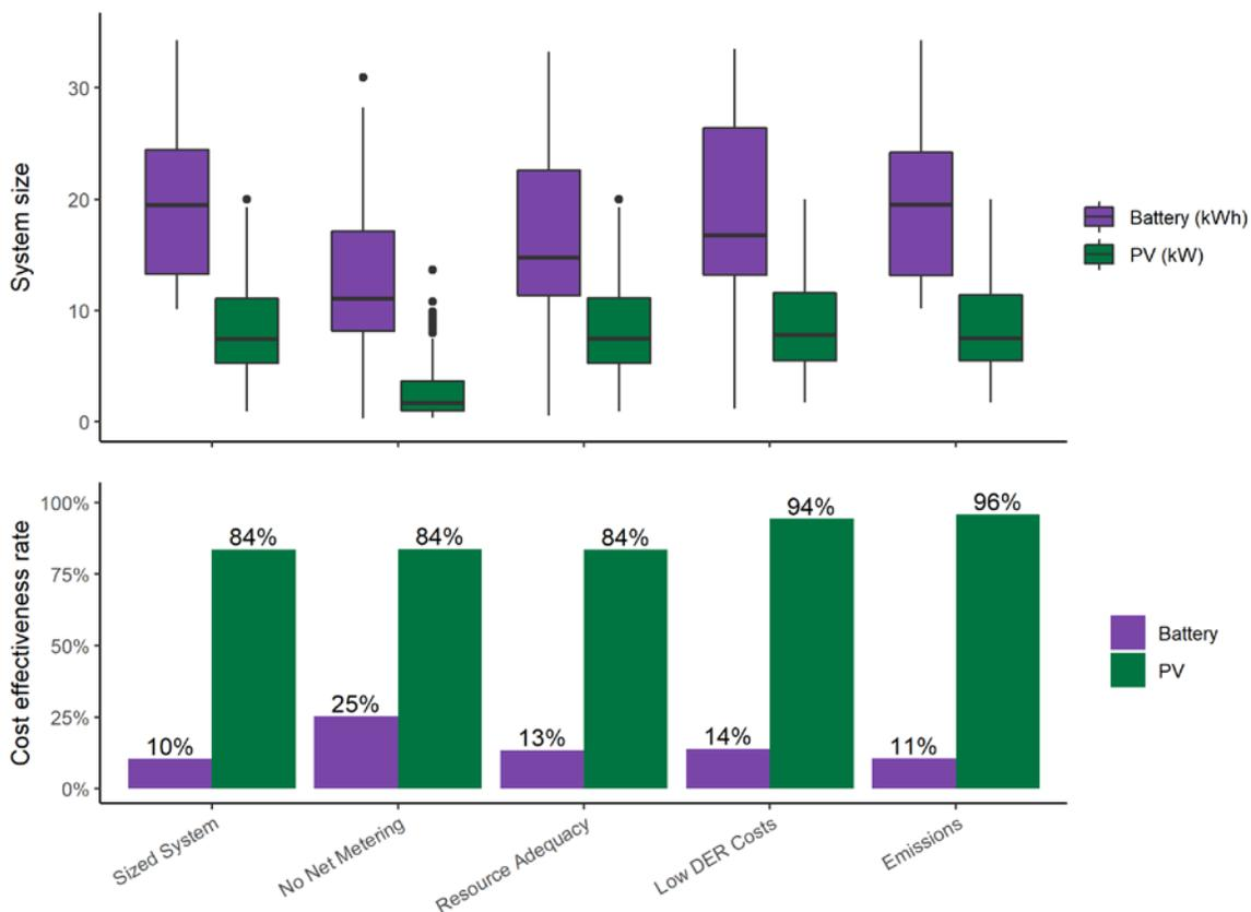
**Figure 17. Cost-effectiveness rate of PV and battery across different scenarios**
