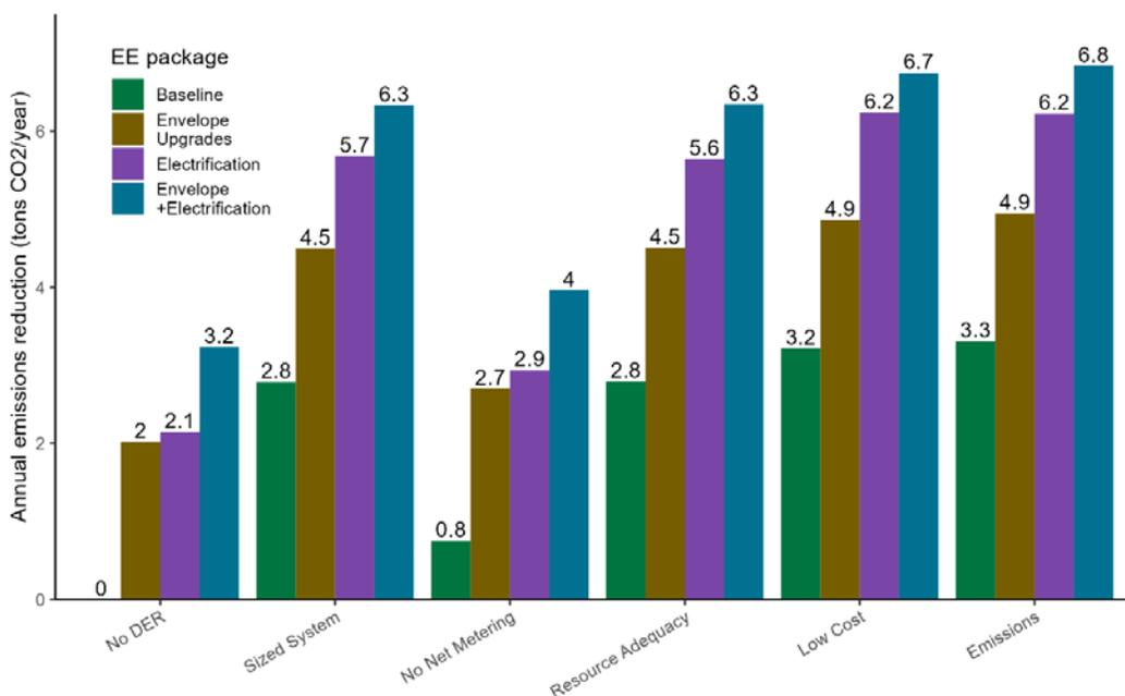
**Figure ES-3. Annual emissions reduction by scenario and energy efficiency upgrade**
