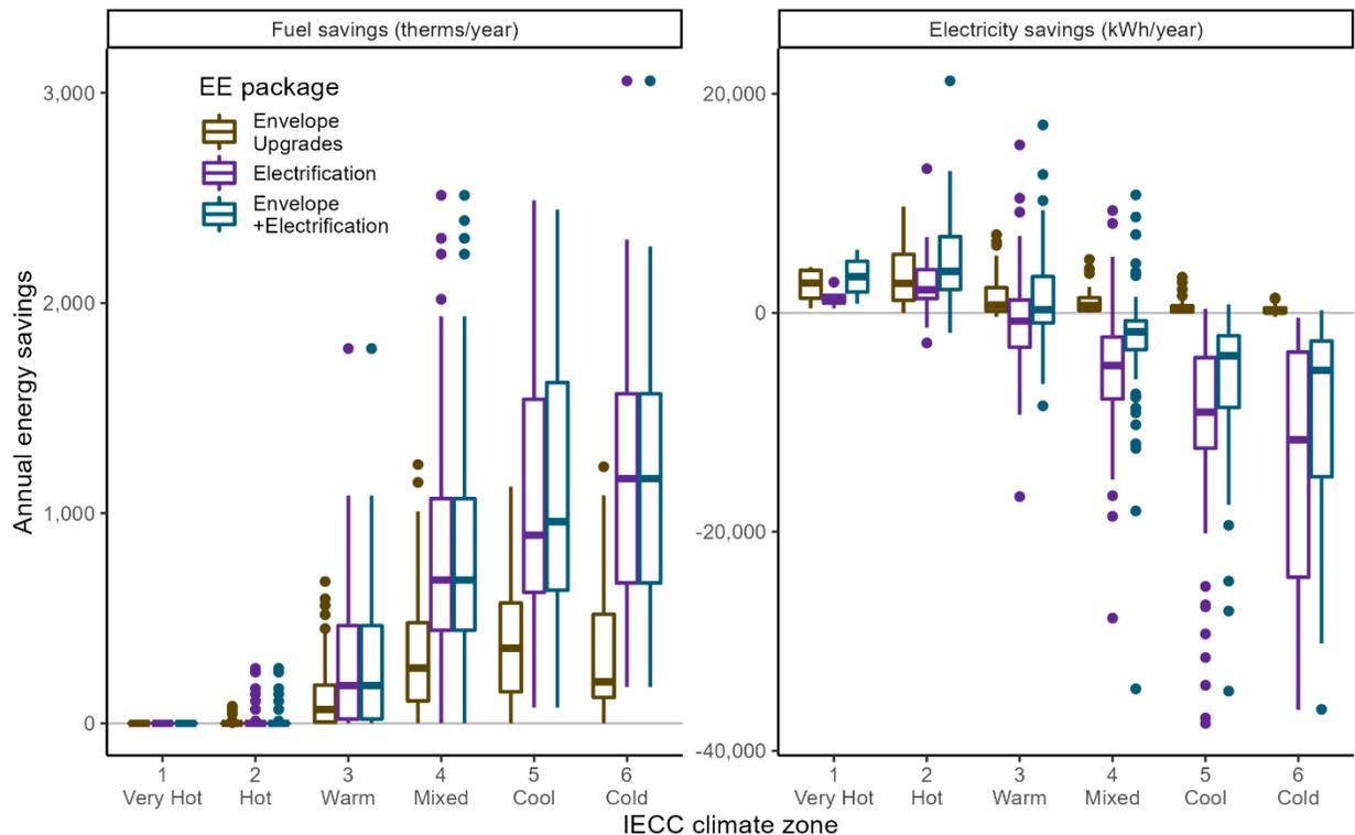
**Figure 10. Annual energy use reduction for each upgrade package, by IECC climate zone**
