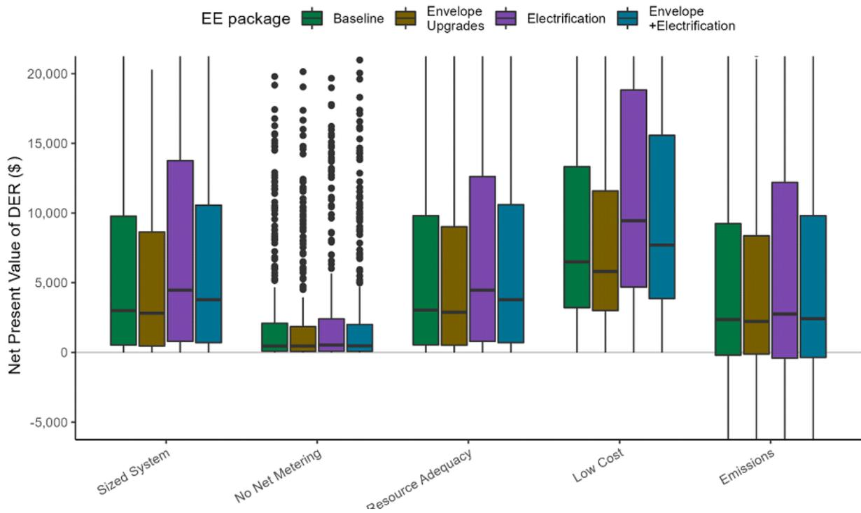
**Figure 22. Average net present value of DER upgrades by scenario and EE upgrade**
