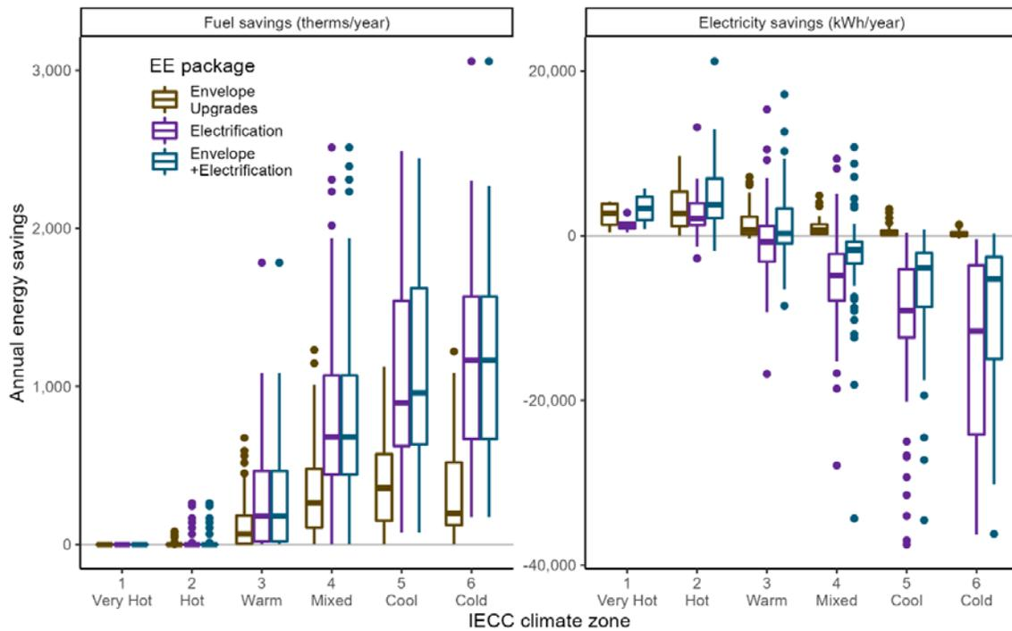
**Figure ES-2. Annual energy use reduction for the three EE upgrades, by IECC climate zone**
