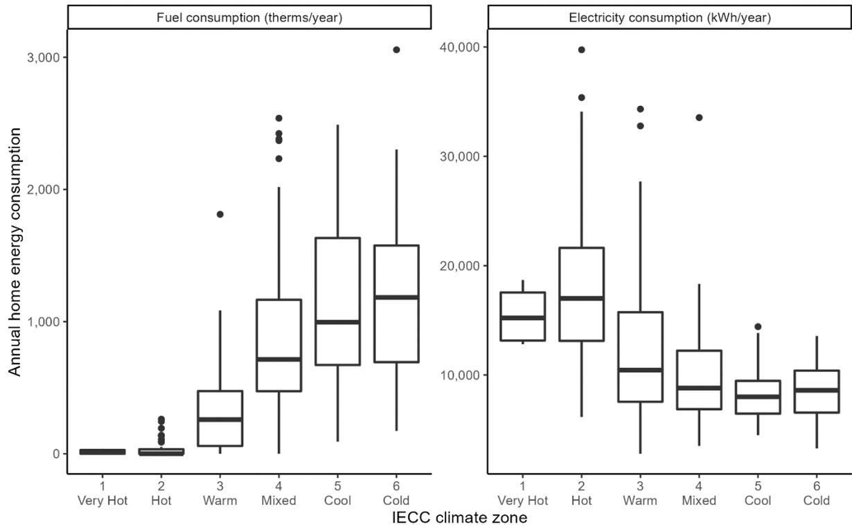
**Figure 7. Annual total energy consumption by energy source and climate zone for baseline housing stock in this study**
