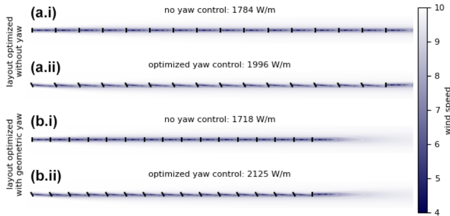
Figure 3. A simple one-dimensional optimization of a 16-turbine wind power plant comparing the performance of the layout optimized without yaw control and the layout optimized with geometric yaw. Panels (a.i) and (a.ii) show the layout that was optimized assuming no yaw control. Panels (b.i) and (b.ii) show the layout that was optimized using the geometric yaw relationship. Panels (a.i) and (b.i) show the plant and performance for each optimized layout without yaw control. Panels (a.ii) and (b.ii) show these same layouts but with the final optimized yaw angles.
