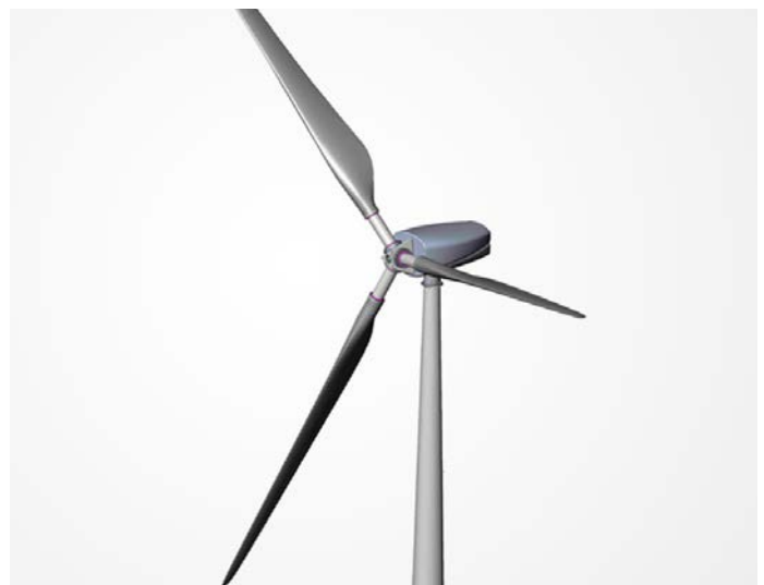
The 60-kW Zephyr 21/60 wind turbine from Windward Engineering uses a low-cost, full-span independent pitch system that can act as a redundant aerodynamic braking system. In this graphic, the wind turbine is shown with its blades pitched in its parked (brake) orientation. Image from Dean Davis, Windward Engineering
