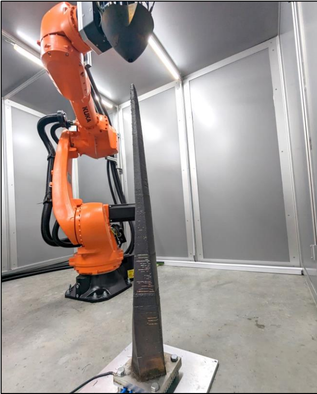
Fig. 13. The structural box spar print, complete with the Kuka/Meltio LMD system (photo by Phil Barden, Ai-Build).
