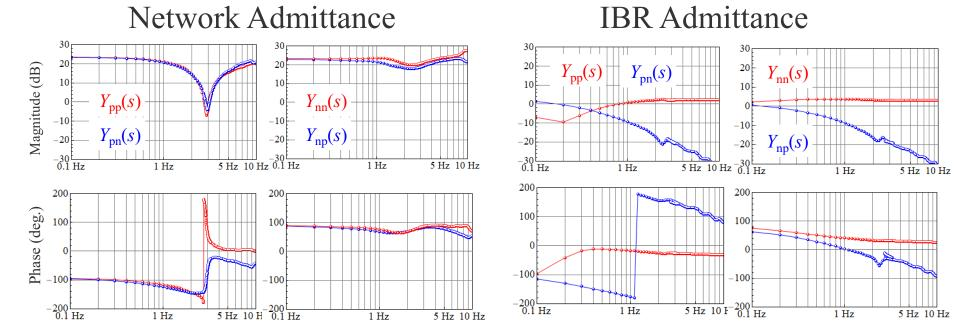
**Impedance Scan Tool Separates the Dynamics of an IBR from the Network**
