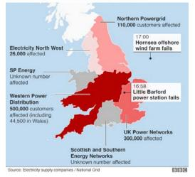
700-MW Hornsea Offshore Wind Plant Contribute d to UK Blackout in August 2019 Plant reactive power output had 8.5 Hz oscillations following a small (2%) step change in voltage
