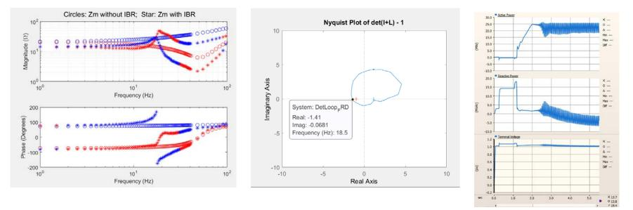
• Plant is unstable stable – confirmed by time-domain simulations (17.4 Hz)
