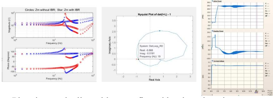
• Plant is marginally stable – confirmed by time-domain simulations (19.4 Hz)
