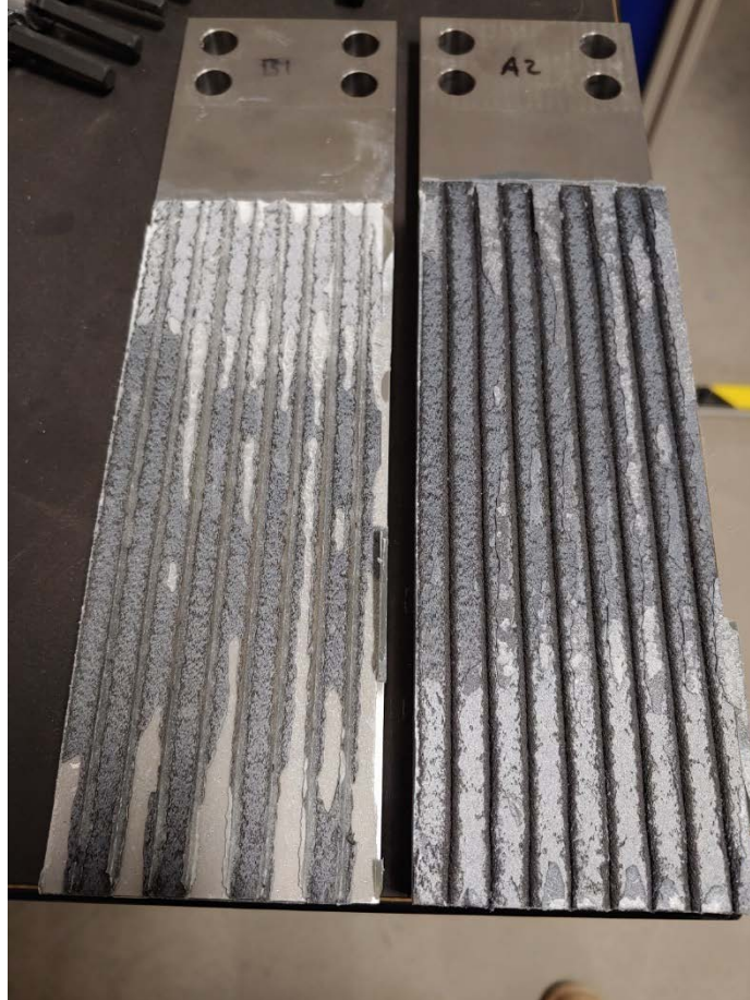
Figure 30. 3D-printed thermoplastic coupon specimen ABSCCF20-3 after loading to failure. Photo by NREL
