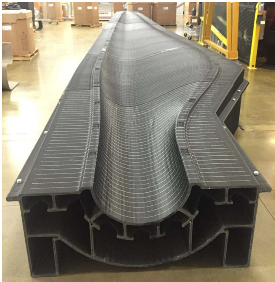
Figure 1. The 13-m 3D-printed wind turbine blade mold. Image from Oak Ridge National Laboratory
