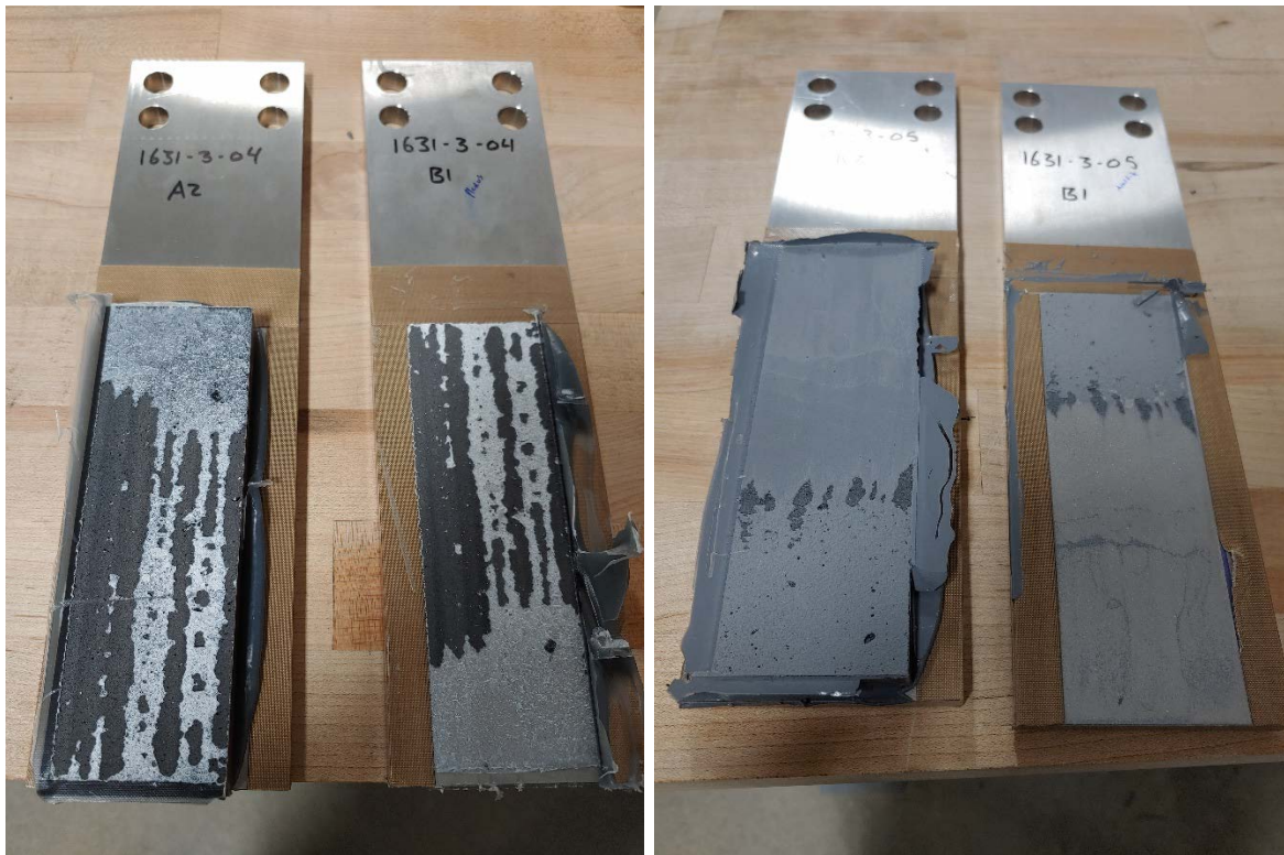
Figure 33. 3D-printed thermoset coupon specimens 1631-3-04 (left) and 1631-3-05 (right) after loading to failure. Photo by NREL
