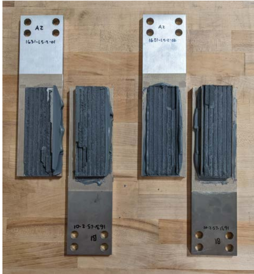
Figure 32. 3D-printed thermoset coupon specimens 1631-LS-2-01 (left) and 1631-LS-2-02 (right) after loading to failure. Photo by NREL
