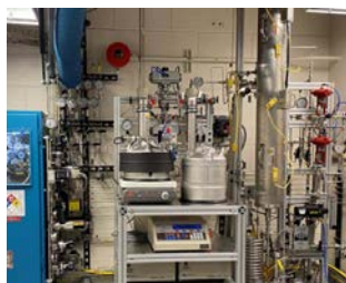
Continuous Hydrotreater (CHT) 10 mL/h Feed
