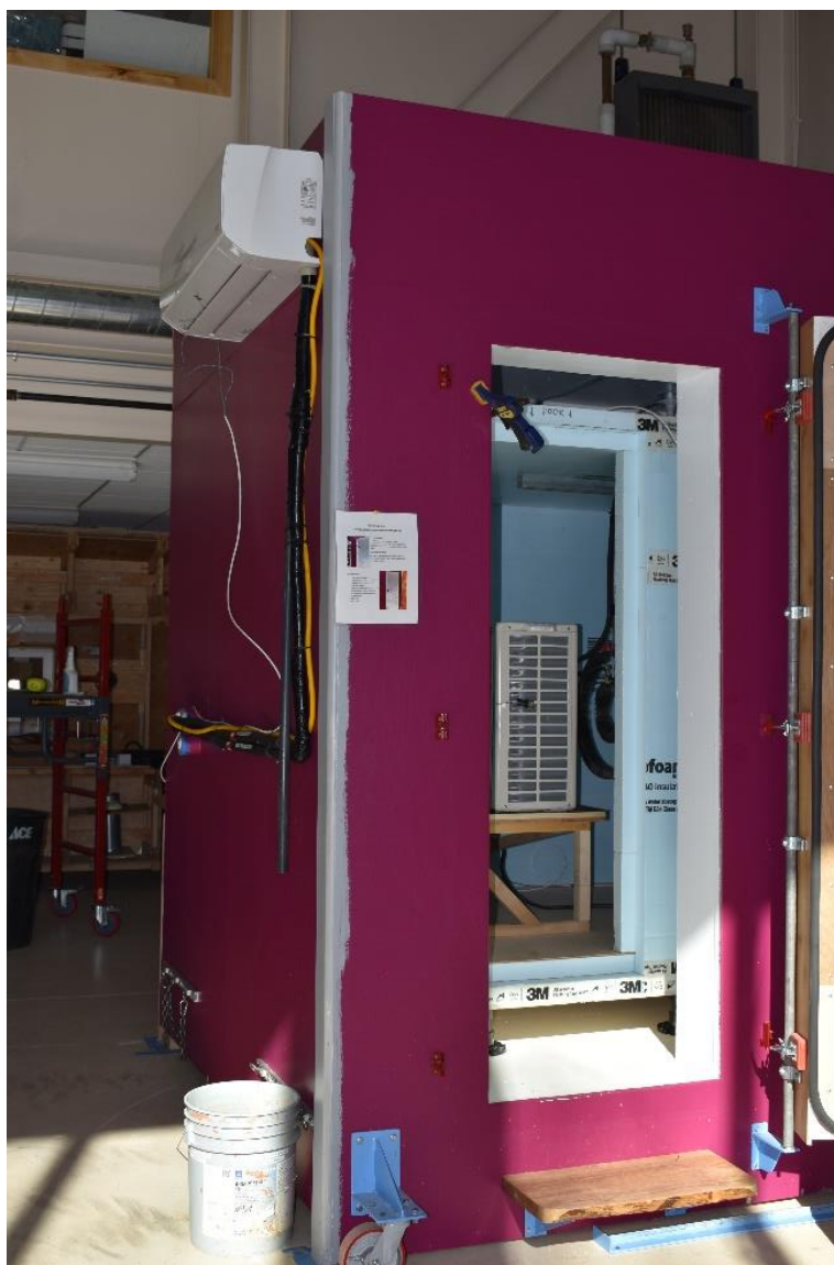
Figure 2. The cold chamber and metering box set up for evaluating ductless ASHPs in the CCHRC laboratory space.
