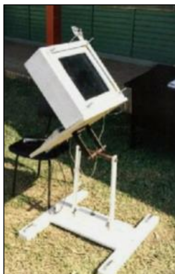
Figure 28. Front View of Fenestration Radiometer Prototype [38].
