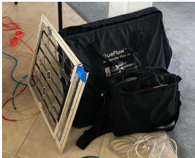
Figure 7. Flow plate used for IDU airflow measurement.
