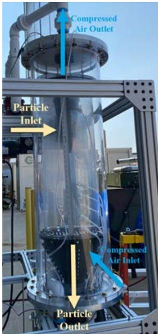
(a) PFB prototype for fluidization test at ambient condition. Photo by NREL.
