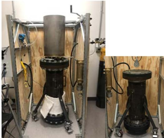
(a) Hot PFB prototype for air/particle heat transfer and fluidization.
