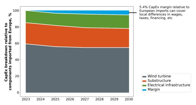
Figure 23. Percent change in component CapEx for wind turbines (including the blades, nacelle, and tower), substructure (including the monopile and the transition piece), and the electrical infrastructure (cables and substations) for scenarios with expanding domestic manufacturing capacity between 2023 and 2030
