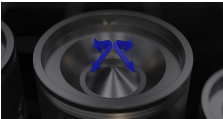
Figure 1: Visualization of the piston-bowl geometry used in the Pele simulations. EBs are used to represent the piston-bowl surface. Fuel is injected at four discrete points at the top of the domain as indicated by the blue arrows.
