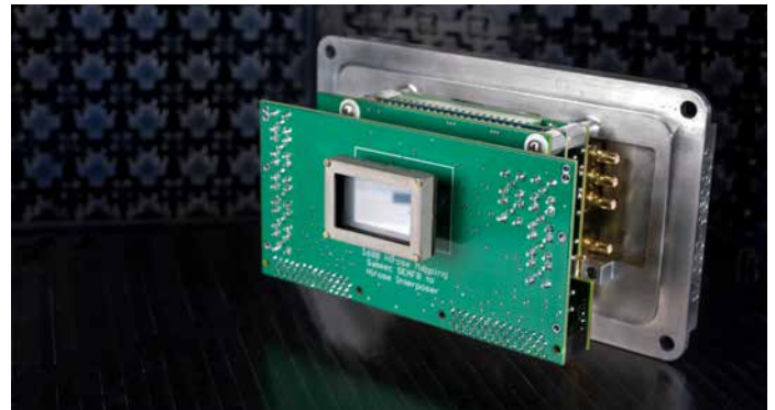
A UXI SNL Z-Machine camera system. Photo by the UXI program, SNL.
