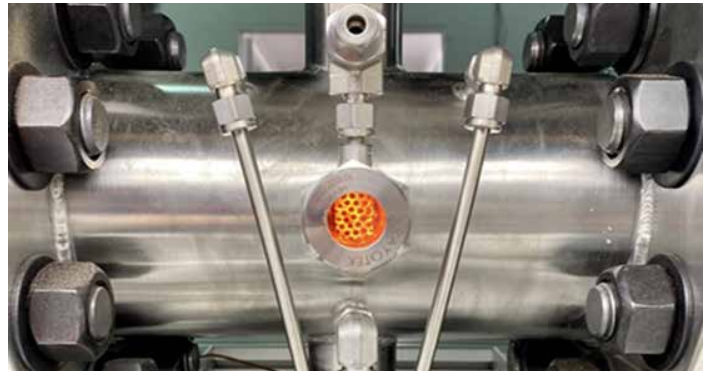
To capture the natural gas instead of burning it, the Catalysis/MAC team uses a microwave reactor, which is an electric-based process to convert the methane into a higher-value chemical, called BTX, commonly used in plastics manufacturing and to create other chemicals. Photo from Catalysis/MAC
