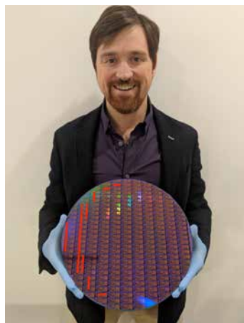
Iris Light founder Chad Husko holding a 12-inch (300-mm) silicon wafer composed of hundreds of chips. Iris Light on-chip lasers are made by depositing proprietary photonic ink onto the surface of a pre-patterned wafer like the one shown here. Photo by: Mary Reid Ervin.
