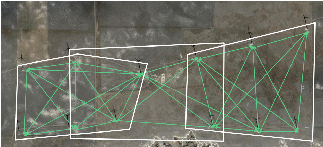
Figure 32. Wind-plant-scaled AT array supporting acoustic transducers on wind turbine nacelles. White regions indicate nested and overlapping retrieval areas.
