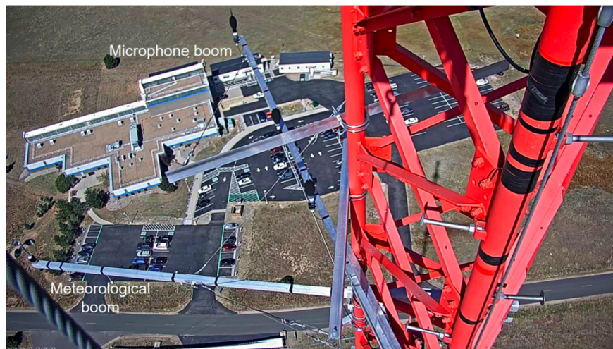
Figure 28. M5 met mast at the NREL Flatirons Campus showing a microphone and meteorological boom from the Kamrath et al. (2021) study.
