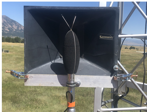
Figure 11. Microphone affixed to speaker aperture for latency test at Station 8.
