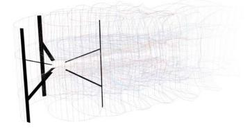
This visualization simulates the flow around XFlow Energy's 25-kW wind turbine. This simulation was made possible with assistance from the National Renewable Energy Laboratory during XFlow's 2019 Prototype Design Development Competitiveness Improvement Project award. *Photo Image by Ian Brownstein, XFlow Energy*
